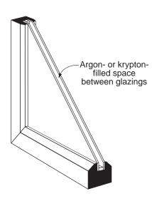
Addition of a second pane to a window assembly doubles the thermal resistance. If a third or fourth pane is added, the thermal resistance also increases, but with a diminishing effect. The trade-off with multiple panes is that while thermal resistance is increased with each pane, visible light transmittance decreases as well as the solar heat gain in the winter months. In addition, more panes also add to the initial cost which may not be recovered over the life of the window.
