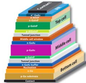
A multi-layered triple-junction solar cell designed to absorb different solar photons.
