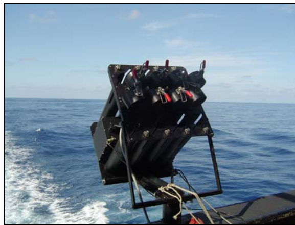
Autolauncher installed on the Horizon Hawaii
