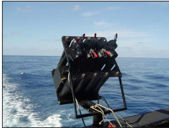
Autolauncher installed on the Horizon Hawaii
