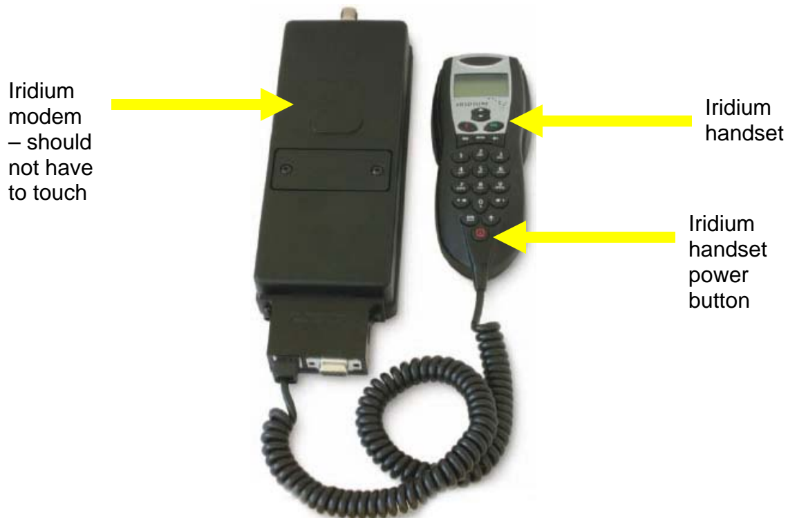
Figure 11. Iridium modem and handset
