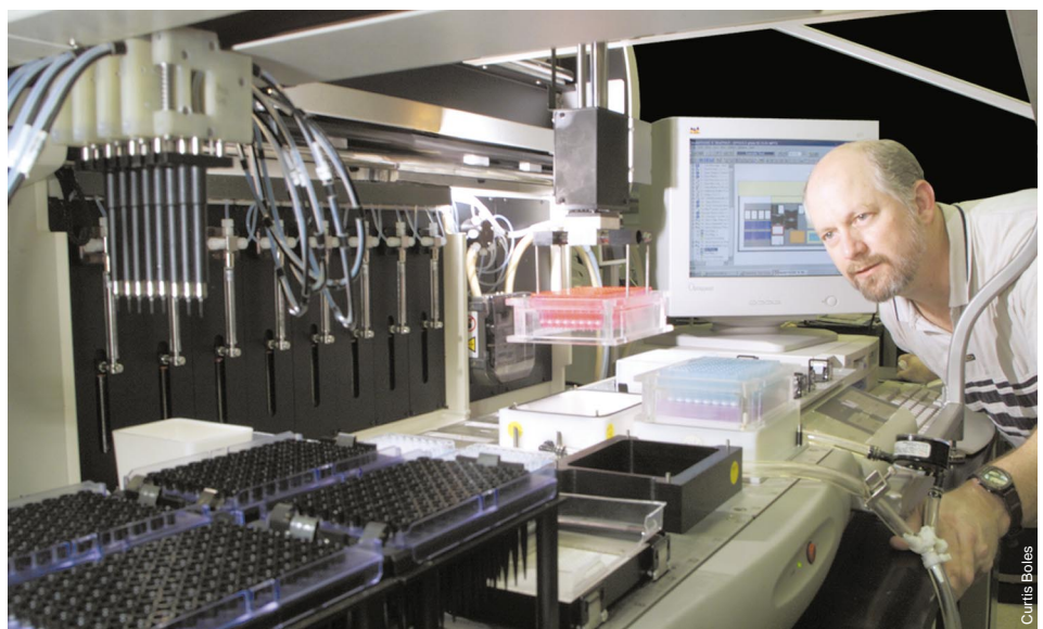
Peter Hoyt checks the operation of the Packard multiprobe liquid-handling system and mechanical gripper. This state-of-the-art robotic tool is used to prepare samples (e.g., cloned DNA) for use on microarrays to analyze gene expression.
