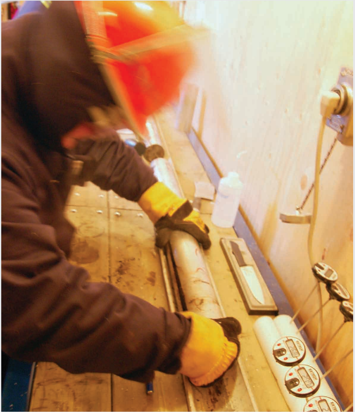
Processing a sediment core from a methane hydrate stratigraphic test well, Mt. Elbert, Alaska's North Slope, Prudhoe Bay.
