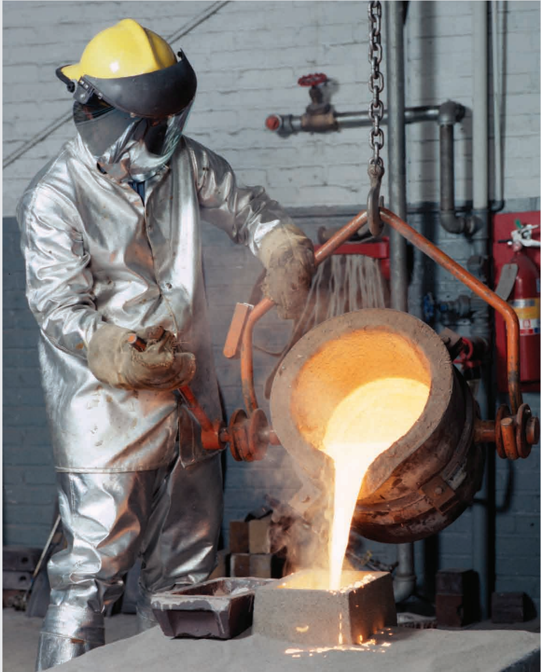
Pouring a cast steel P-900 hatch for the Bradley Fighting Vehicle.
