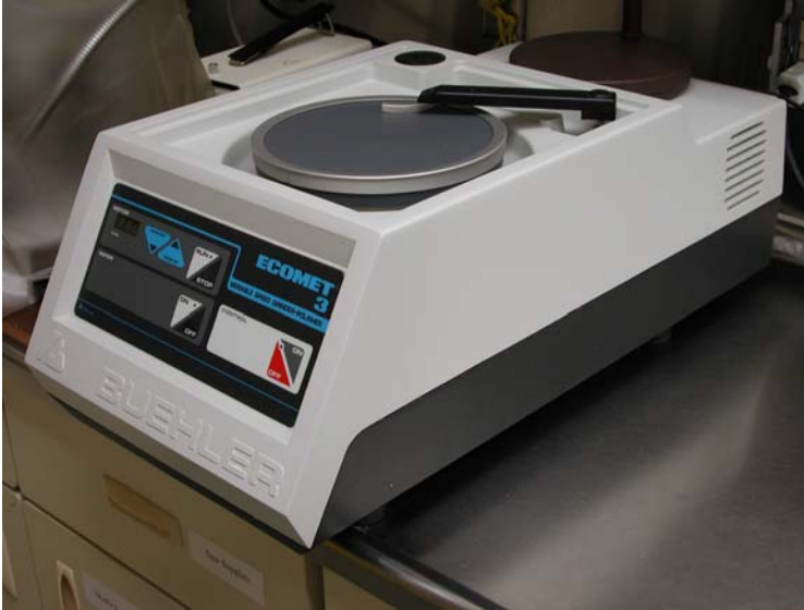
Fig. 10. Buehler Ecomet table sander for sanding and polishing mounted thin sections.
