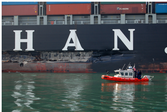
Damage to port side of the vessel. Photo courtesy of U.S. Coast Guard.
