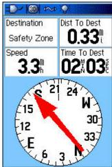
Press **Page** until the **Compass** page appears (left). The **Compass** page features a "compass ring" and four user-selectable data fields. The **Compass** page illustrated at left indicates that:
