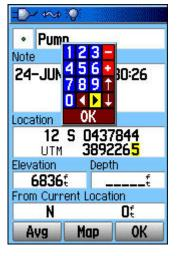
Waypoints can also be created "from scratch". For example, handwritten coordinates for a pump's location can be manually entered to create a new waypoint for the pump. Remember that the receiver's **Position Format** and **Map Datum** must be set to match the coordinates' **Position Format** and **Map Datum** prior to entering the coordinates.
