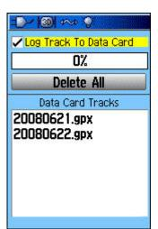
The GPSMAP76CSx has a micro-SD card that can hold a prodigious amount of GPS data. If users are on an extended project with no regular opportunity to download their data, they could have each day's active track log automatically transferred to the micro-SD card in GPX format. The GPX format is recognized by most GPS processing software, including DNRGarmin.
