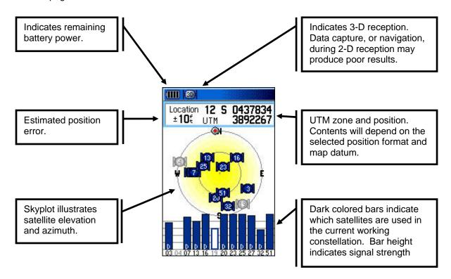
**WAAS** - WAAS (Wide Area Augmentation System) is a form of satellite-based real-time differential correction. If WAAS correction is enabled by the user, it may improve position quality by several meters.
