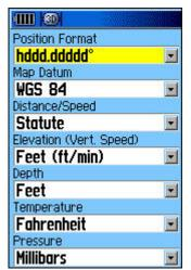
**Position Format And Map Datum** - Garmin GPS receivers capture and store positions as decimal degrees of latitude and longitude referenced to the WGS84 datum. Although users can set how GPS positions are displayed on-screen, those settings have no effect on how the GPS positions are actually captured, or stored, internally.
