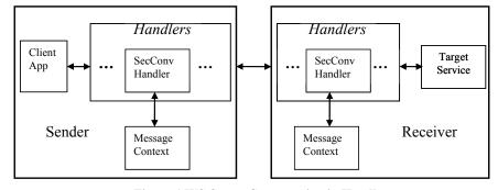
Figure 1 WS-SecureConversation in Handlers
