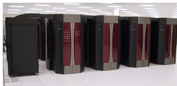
Figure 1: Front view of 256-MSP, 8-cabinet Cray X1 at ORNL's Center for Computational Sciences.
