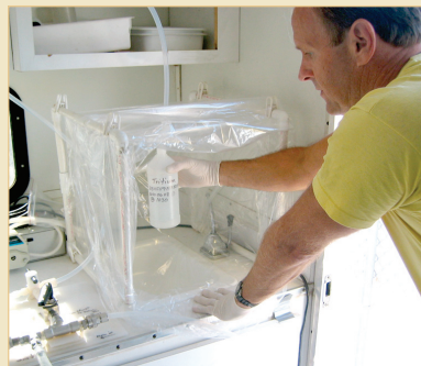
Processing of ground-water samples in a mobile laboratory, including samples for analysis of tritium. (photograph by Carmen Burton, U.S. Geological Survey)
