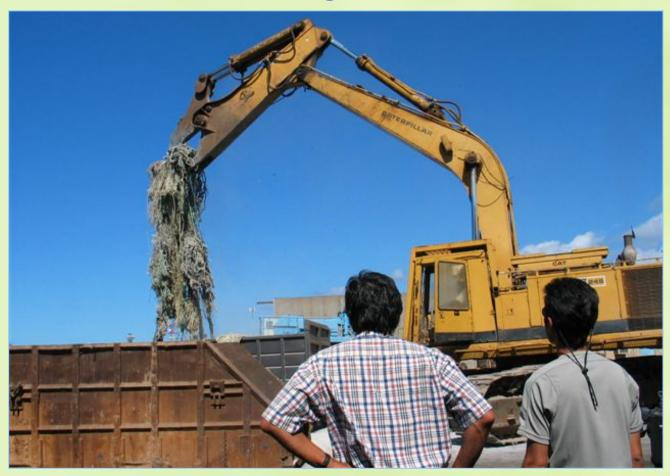
\* At the HMR baseyard, specialized equipment cuts the mountains of net into pieces small enough to flow into the conveyor belts of H-POWER, Honolulu's garbage-to-energy plant.
