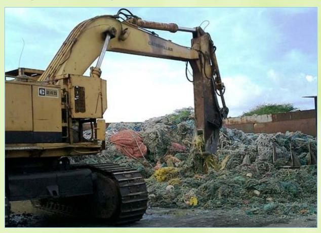
\* Although the cutting equipment is designed to chop up auto bodies, cutting the tangled net proved much more difficult. Brand-new blades must be used to cut through layers of hemp, nylon, and plastic.
