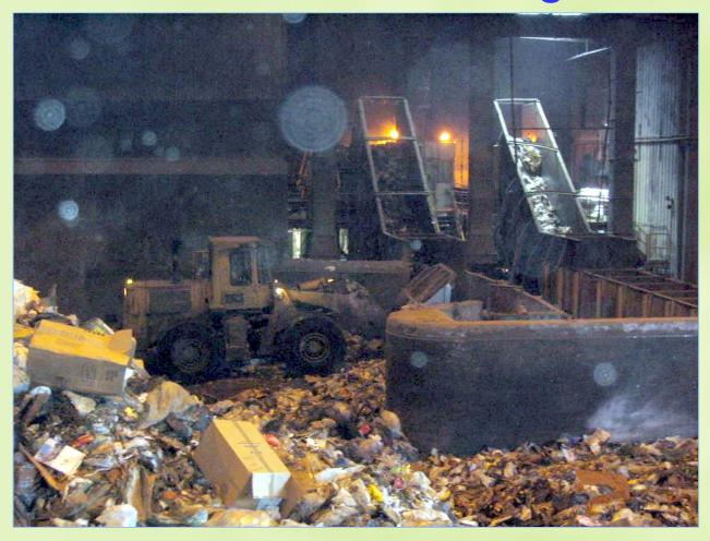
\* H-POWER's conveyor belts, right, can only accommodate smaller sizes of fibrous materials such as net. Large sizes snag and shut down the operation.
