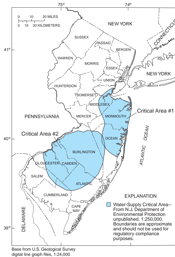
Figure 2. Location of Water-Supply Critical Areas in New Jersey. These areas were designated to help control the decline in water levels in some of the confined aquifers. (From Watt, 2000)
