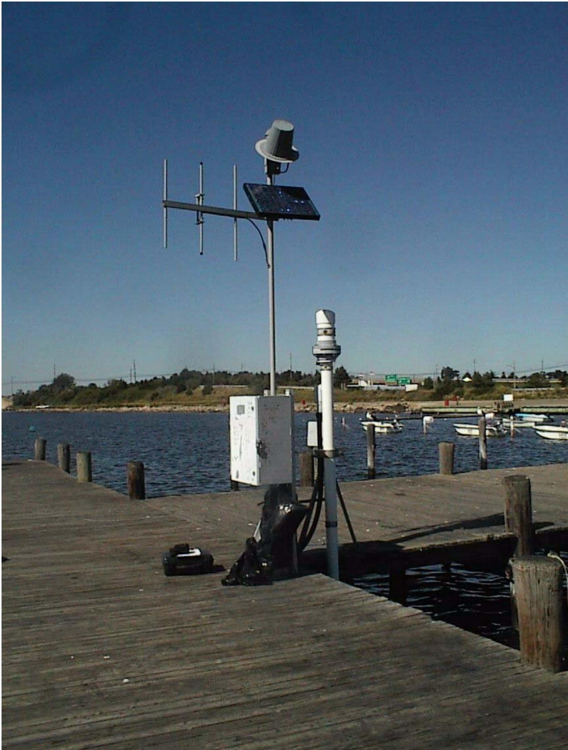
Figure 19. U.S. Geological Survey tide gage continuously monitoring the elevation of water surface at Barnegat Bay at Seaside Heights, NJ. Photograph taken by Peter B. Reilly, 2002.
