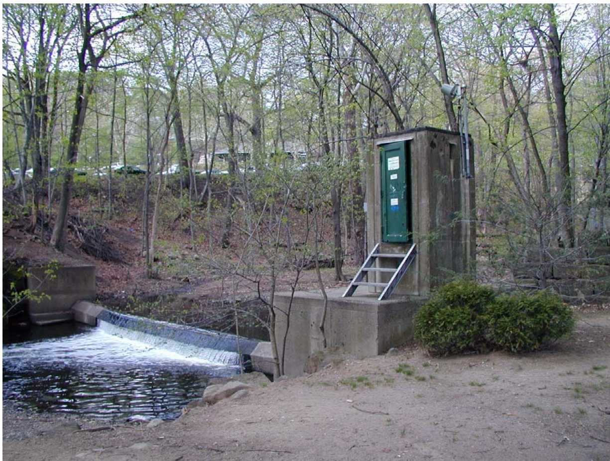
Figure 15. U.S. Geological Survey gage continuously monitoring the stage of Hohokus Brook at Ho-Ho-Kus, NJ. Photograph taken by Richard W. Edwards, 2002.
