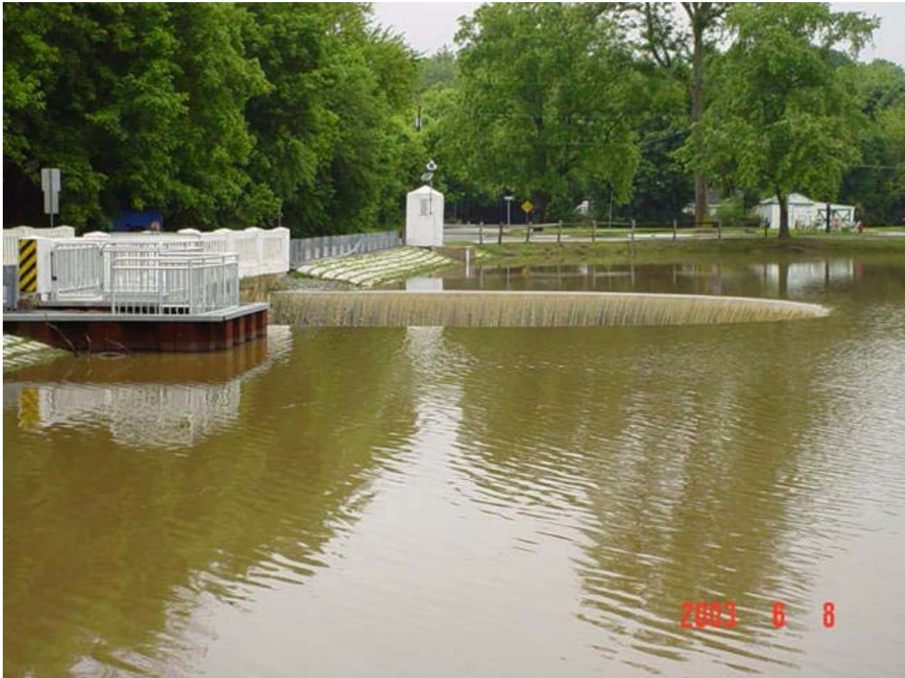
Figure 24. U.S. Geological Survey gage continuously monitoring the stage at Salem River at Woodstown, NJ. Photograph taken by Blaine T. White, 2003.
