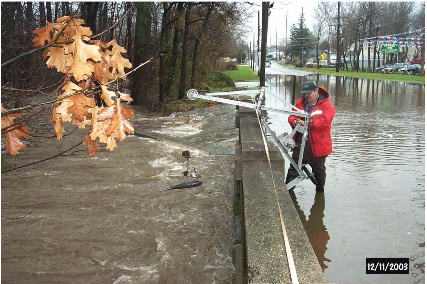
Figure 23. U.S. Geological Survey hydrographer, Guerino Centinaro, measuring flow at Mantua Creek at Pitman, NJ. Photograph taken by Joseph Orlins, Ph.D. (Rowan University) 2003.
