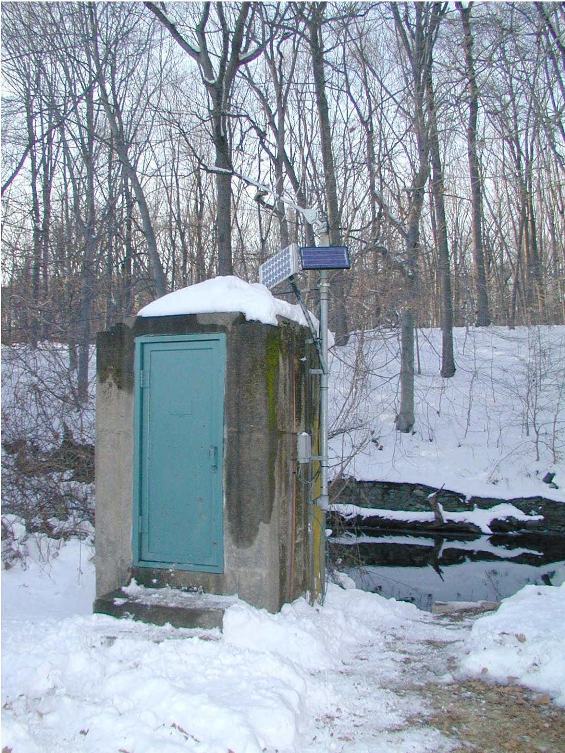
Figure 14. U.S. Geological Survey gage continuously monitoring the stage of the Rockaway River below reservoir at Boonton, NJ. Photo taken by Richard W. Edwards, 2003.
