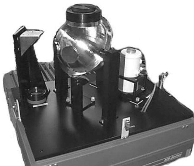
Figure 15. Photograph of Bomem MB-100 w/gold sphere. The gold integrating sphere is mounted in the standard sample compartment area above the FT-IR. The sphere's entrance port can be seen on its left side facing the focusing mirror. The larger port cover next to it can be removed for separation of diffuse and specular (reflectance) components. The sample is loaded and rotated from the top of the sphere and located at its center. An ellipsoidal mirror (out of view) is used to focus the small exit port underneath the sphere onto the detector (white dewar at the right) detector. The reference measurement is made, after rotation of the sample, with a reference standard mounted back-to-back with the sample. (Reproduced by permission of ABB Bomem Inc.)
