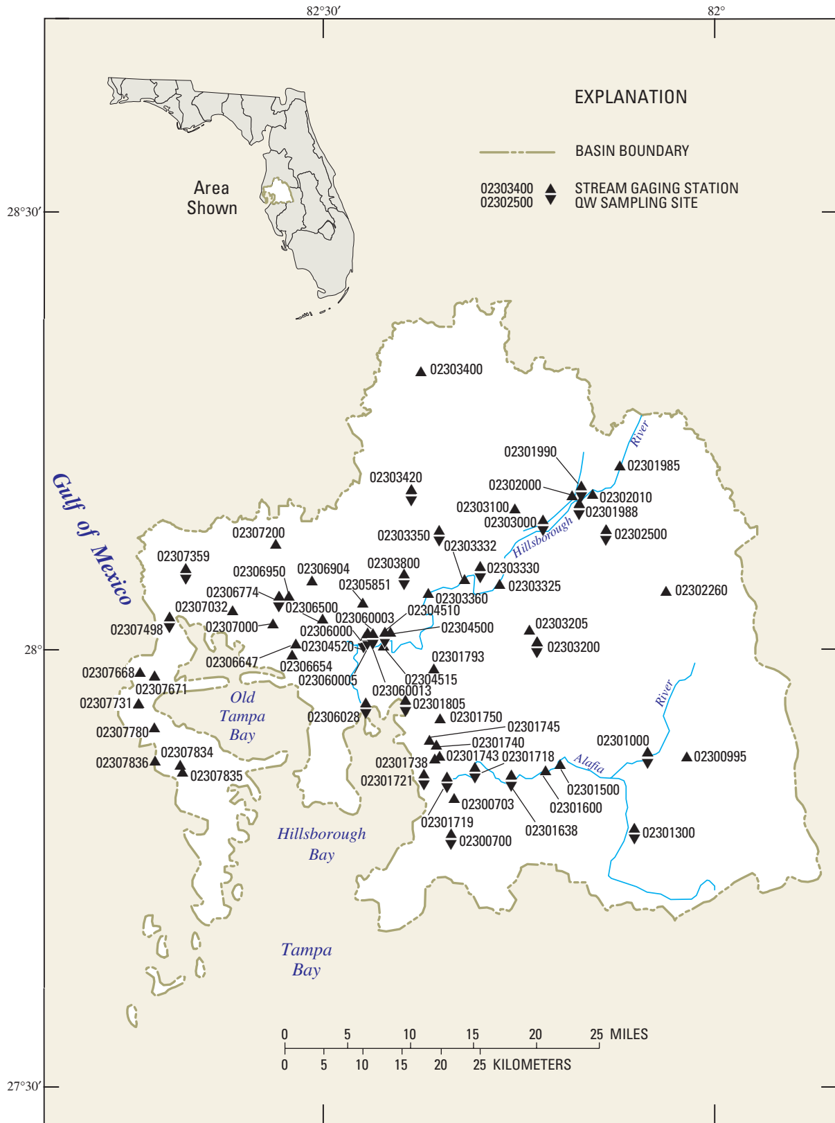
Figure 13.--Location of stream gaging stations in the Alafia and Hillsborough River Basins, Tampa Bay and Coastal area.
