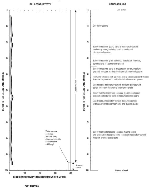
Bulk conductivity, in millisiemens per meter, April 26, 2005. Shaded area represents range of measurement in bulk conductivity logs collected from January 9, 1995 to April 26, 2004. Bracket represents the interval for which the
