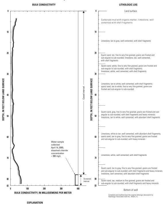
Bulk conductivity, in millisiemens per meter, April 14, 2005. Shaded area represents range of measurement in bulk conductivity logs collected from April 13, 2000 to April 26, 2004. Bracket represents the interval for which the
