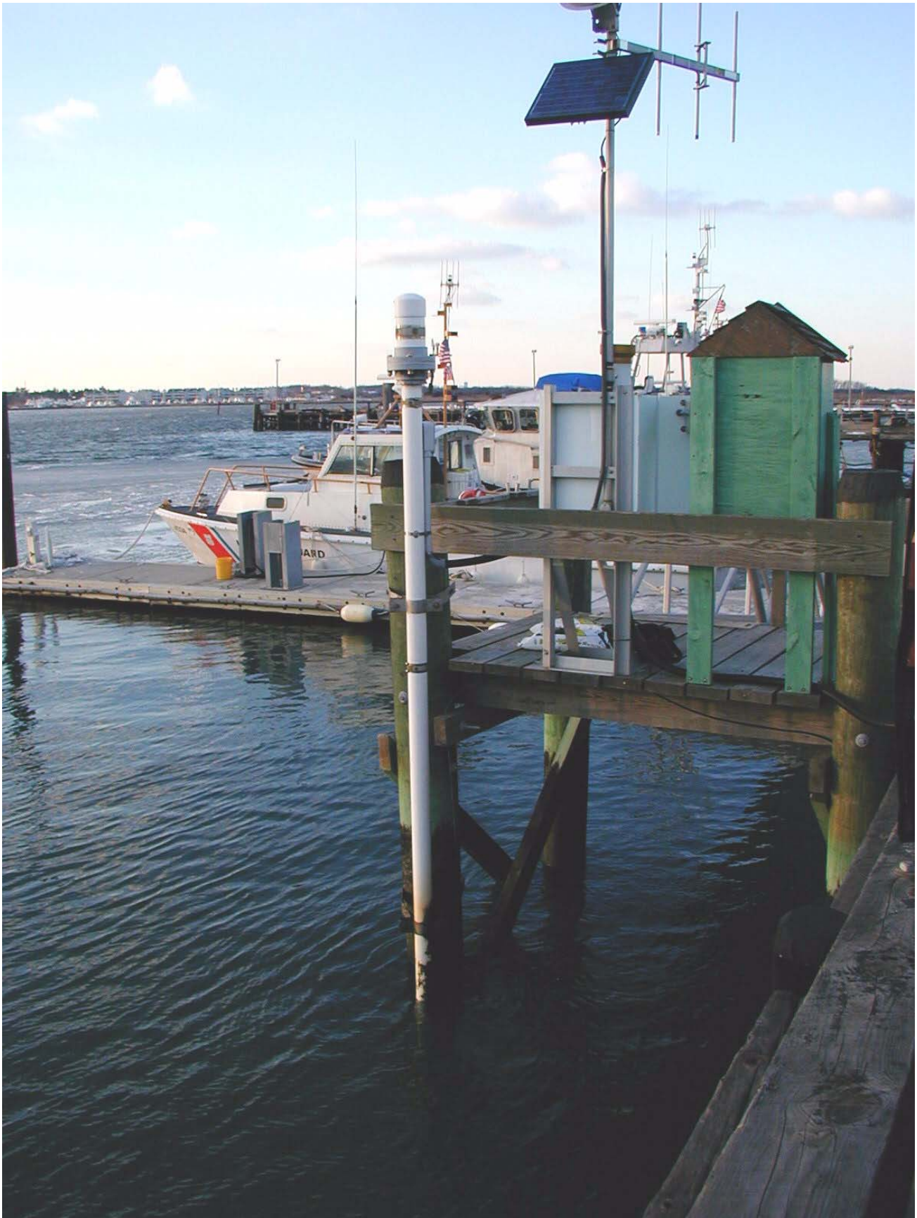
Figure 17. U.S. Geological Survey tide gage continuously monitoring the elevation of water surface at Cape May Harbor at Cape May, NJ. Photograph taken by Peter B. Reilly, 2002.
