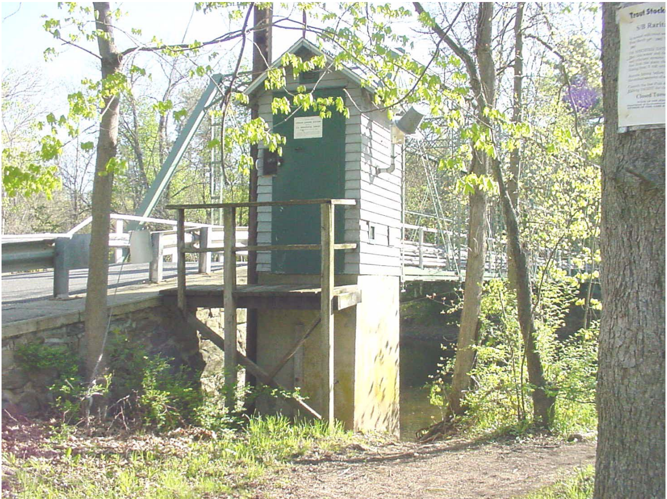
Figure 15. U.S. Geological Survey gage continuously monitoring the stage of the South Branch Raritan River at Stanton, NJ. Photograph taken by Blaine White, 2002.
