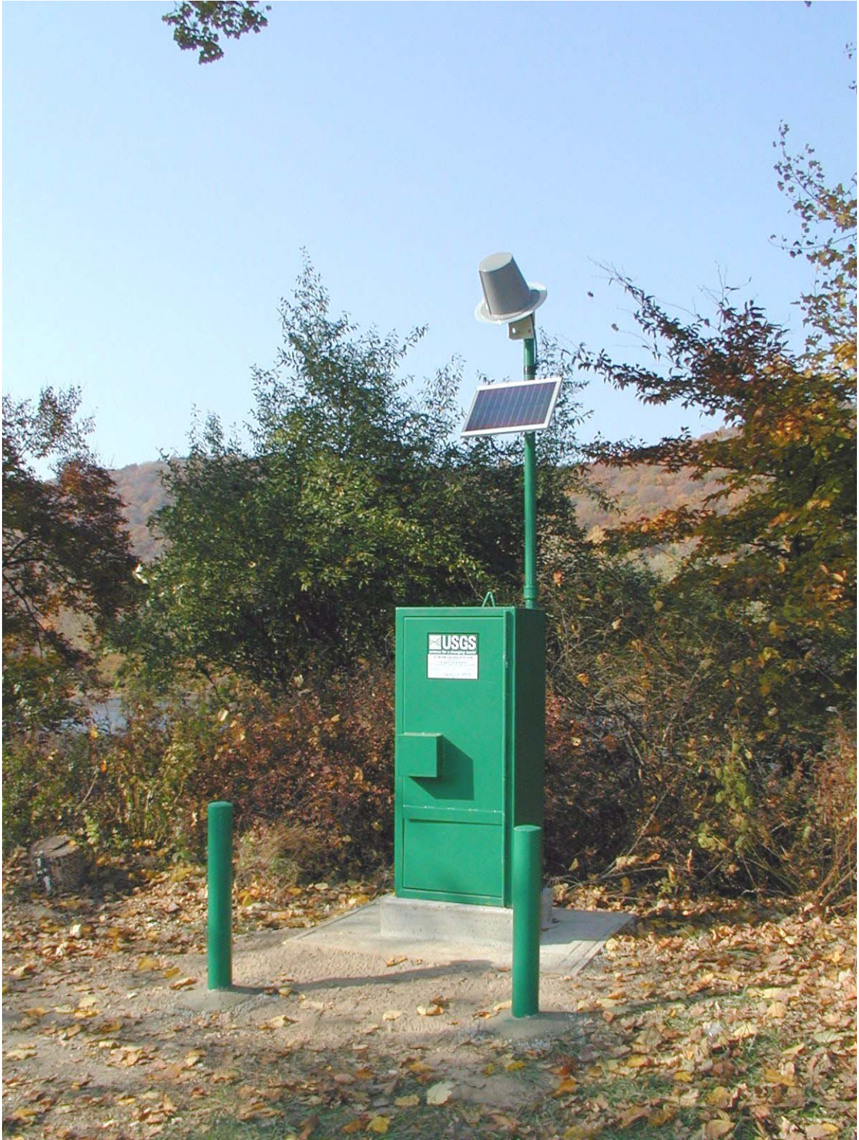
Figure 19. U.S. Geological Survey gage continuously monitoring the stage of the Delaware River near Delaware Water Gap, PA. Photograph taken by Rick Edwards, 2001.
