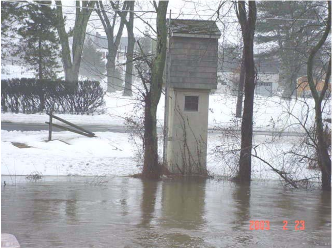
Figure 16. U.S. Geological Survey gage, in foreground, continuously monitoring the stage of the Millstone River at Blackwells Mills, NJ. Photograph taken by Jason Shvanda, 2003.
