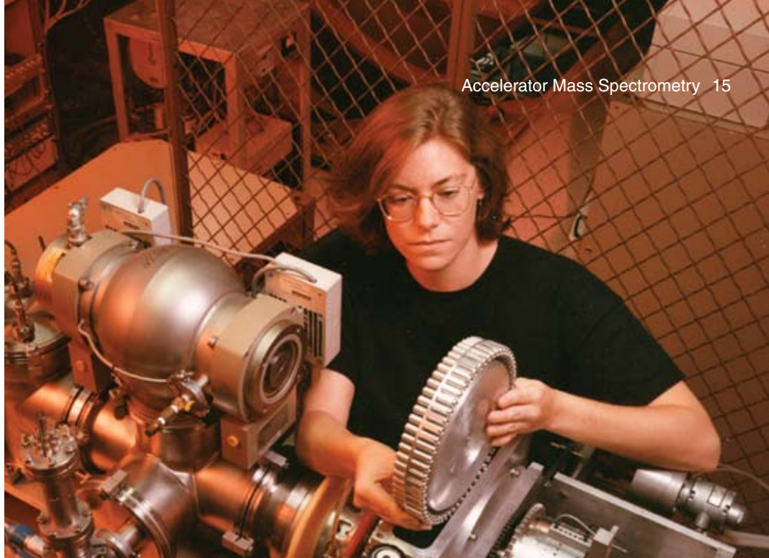
Some accelerator mass spectrometry measurements require that samples be converted to small cylinders of graphite before they are ionized inside the spectrometer. Michale Kashgarian places the sample holder.
