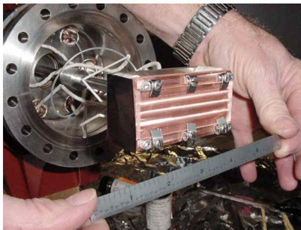
Fig. 2. Large sample mount showing 69-mm \times 29-mm \times 3-mm cleaved LiF target mounted on a heated sample stage capable of being heated to 400^\circ\text{C} .
