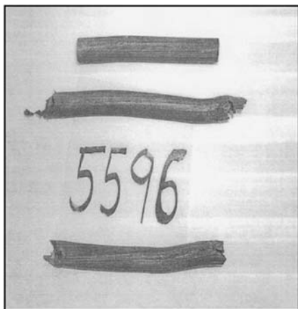
Fig. 1. Photograph of hot-extruded Ti_3SiC_2 in a tantalum-lined 304 stainless steel can. The extrusion products had tears and broke in several pieces.
