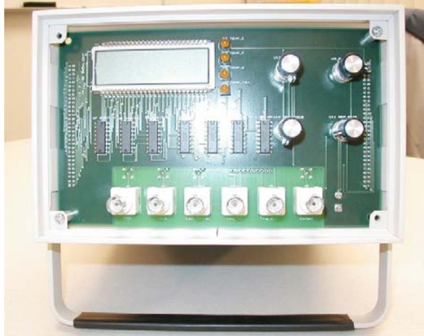
Fig. 1. FPGA-Based Decay Lifetime Measurement Prototype.
