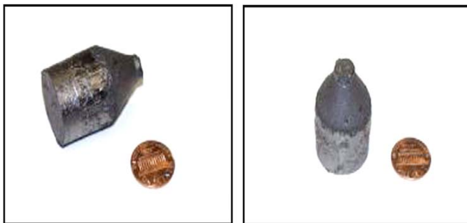
Fig. 2. Photograph of dense Ti_3SiC_2 body after hot-extrusion at 1400^\circ C in a graphite die using a hydraulic press and a graphite furnace.
