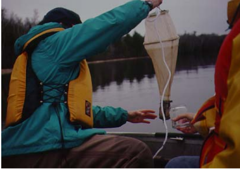
Figure 5. The cone section at the top of a Wisconsin net eliminates some of the water pressure caused by pulling the net through water and makes for a more accurate sample collection.
