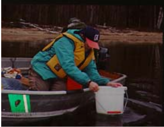
Figure 7. Depending on the quality of the sediment you are collecting, sieving can take a lot of time and energy! Sand and gravel sediment are easy to sieve, but sediment rich in organics and debris will take a lot more time.
