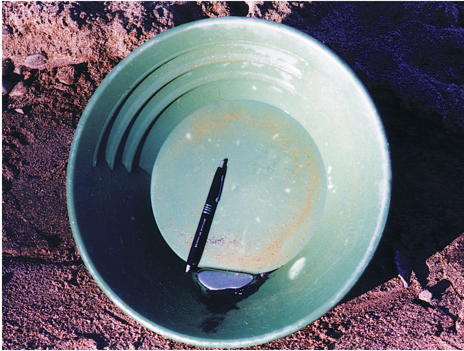
Figure 2. Gold pan with elemental mercury obtained from mercury-contaminated sediments. Such elemental mercury presently remains in sediments and abandoned sluice boxes at sites of historic gold mining in the California Sierra Nevada.
