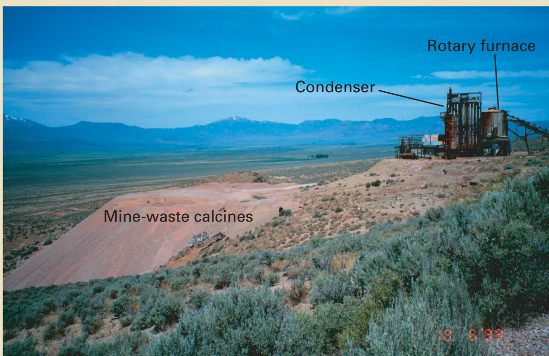
Figure 4. Inactive mercury mine in Nevada. In the rotary furnace, mercury ore was burned producing mercury gas that was cooled, condensed as elemental mercury, and collected.
