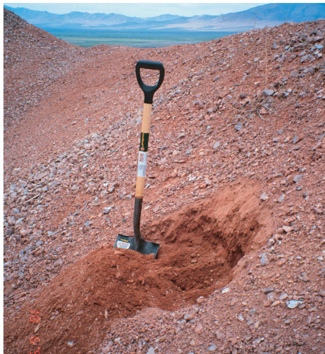
Figure 13. Typical mercury mine-waste calcines. Red-brown character of these mine wastes is a result of presence of iron oxide and fine-grained cinnabar.
