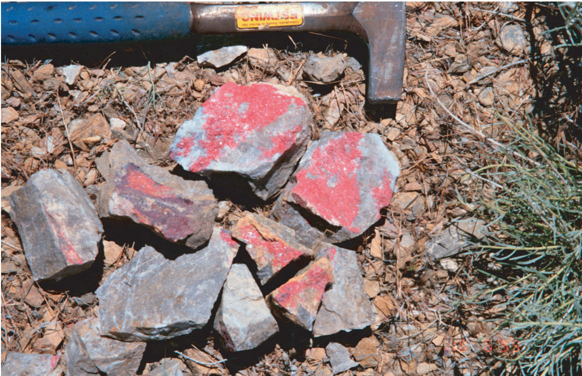
Figure 3. A sample of cinnabar (red mineral), the most common mercury ore in mercury mines worldwide.
