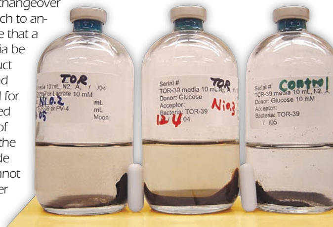
Black powder in NanoFermentation broths with magnets attracting plumes of magnetic particles. The bottles contain various compositions of magnetite.
