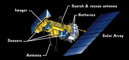
It orbits 14 times a day, about 500 miles above Earth. It passes nearly over the North and South Poles. With Earth rotating below, each POES passes over your area twice each day. Heat sensors measure the temperatures of the oceans, the land, the air, and the clouds.
