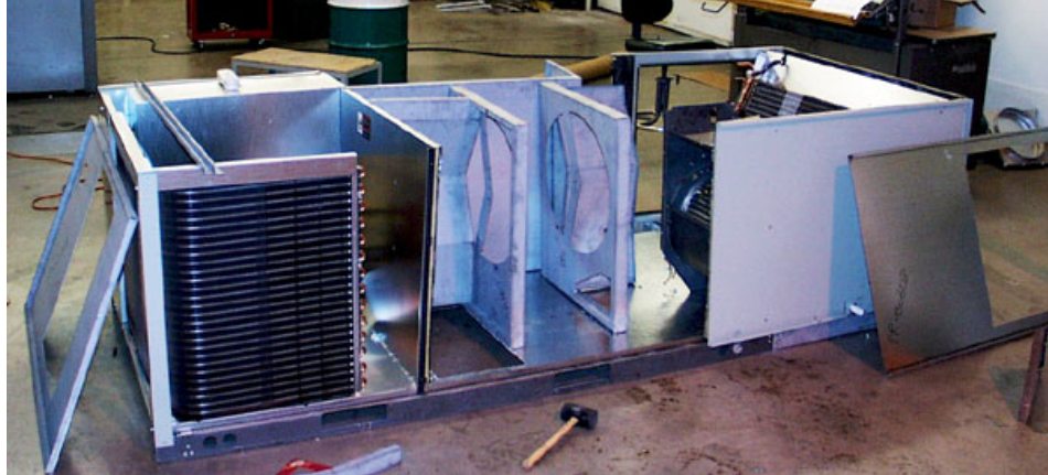
Fig. 8. A photograph of the integrated active desiccant module during assembly, showing how the active wheel section is positioned within the standard rooftop unit.
