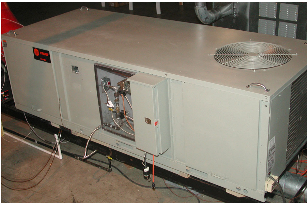
Fig. 9. A photograph of a fully assembled integrated active desiccant module system with the direct-fired regeneration section shown through the glass panel.
