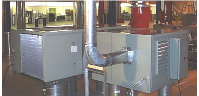
Fig. 2. An add-on active desiccant module and standard rooftop unit in the SEMCO test loop.
