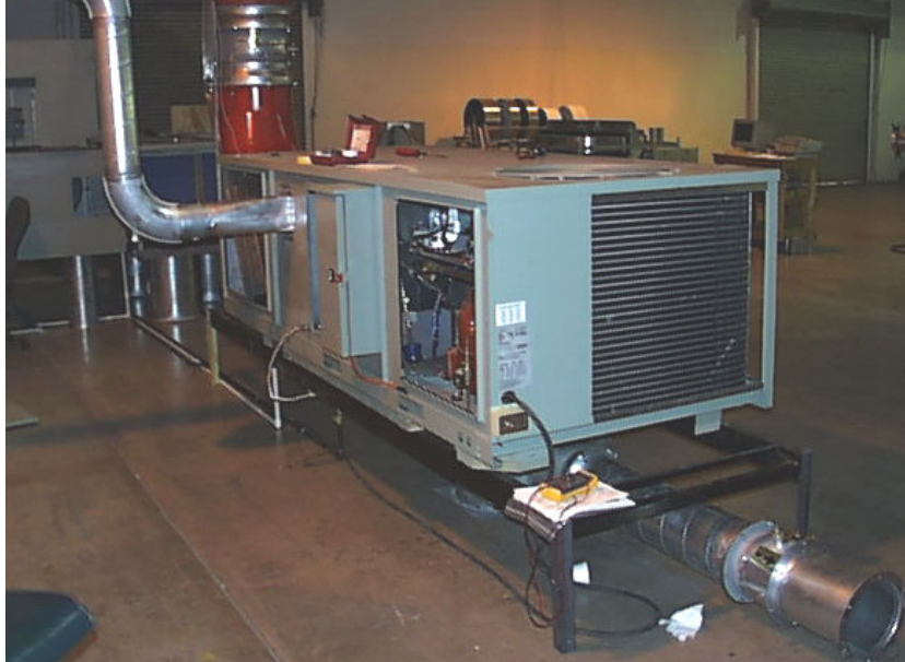
Fig.11. The instrumented integrated active desiccant module system in the SEMCO test loop.
