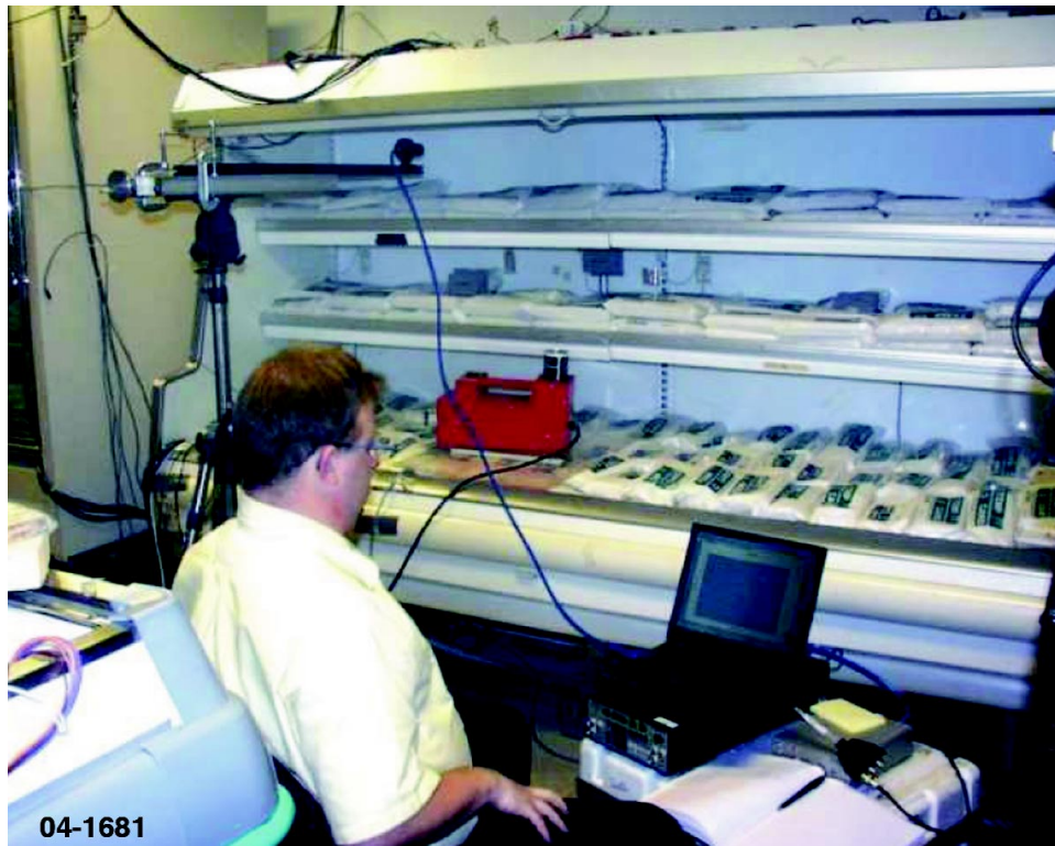
Figure 31. The LDV installation at the DAG of the display case
