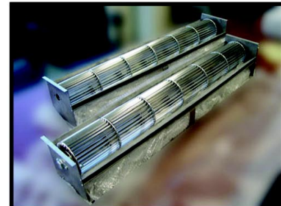
Figure 7. Photographs of the tangential fans and evaporator fan motor
