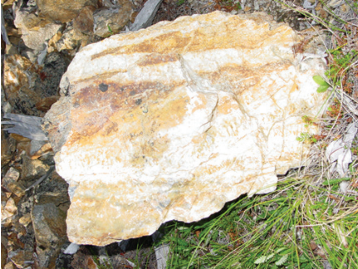
Figure 4. Brecciated stibnite-bearing quartz vein material from Grizzly Bear mine dump (field station 03AD062; lat 64.3569° N., long 144.1929°W.).
