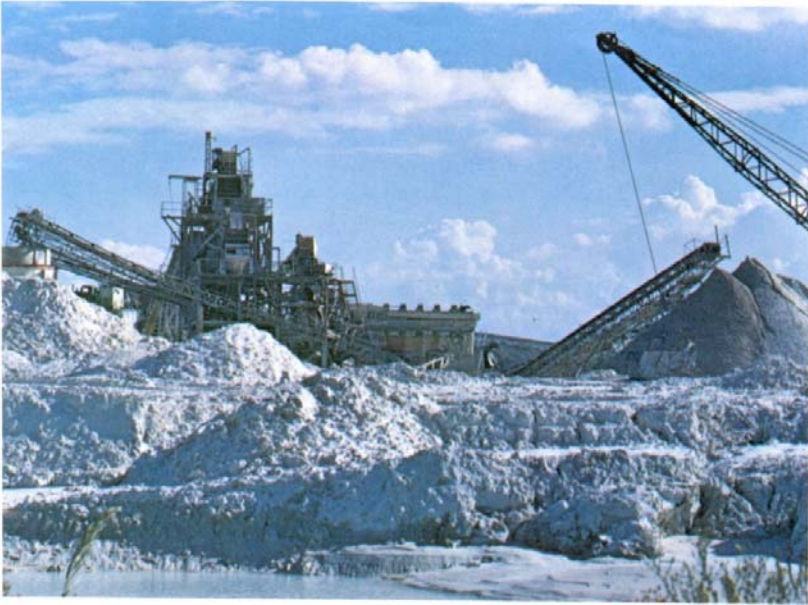
Quarried limestone is crushed to specifications for construction and other uses.
