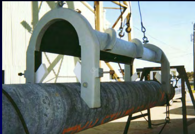
Half strakes for pipelines
