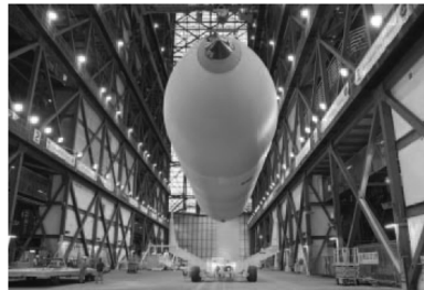
Crews slowly moved an External Tank into the awaiting arms of a transporter in the Vehicle Assembly Building at Kennedy Space Center in October 2004. The Tank then was transferred to NASA's Michoud Assembly Facility in New Orleans, where its foam was replaced with an improved bipod fitting. Afterward, the External Tank was returned to Kennedy, where it waits for return to flight.
