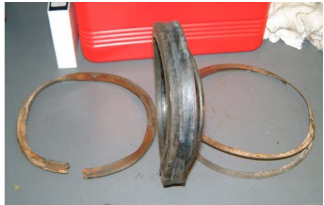
Ram shaft packing after being forced out of the seal pocket by hydrostatic pressure
