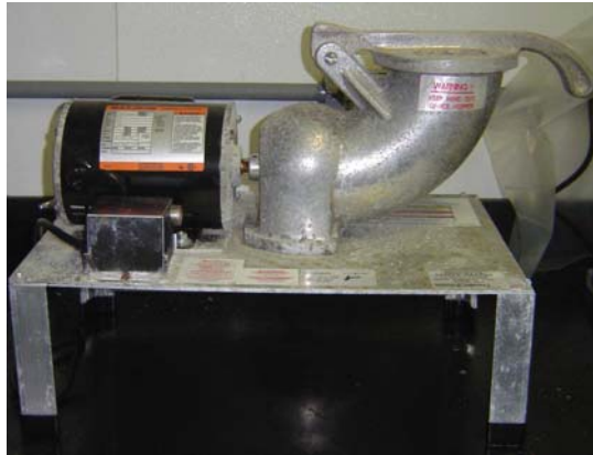
Figure 9. Mechanical ice shaver
