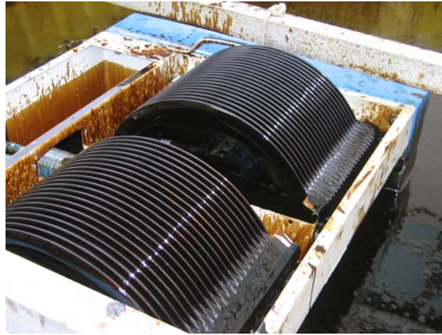
Figure 2. Mini Max® drum skimmer. Standard drums were replaced with grooved drums and a matching cleaning blade.
