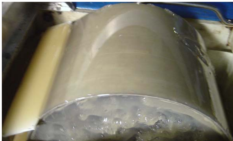
Figure 36. Flat drum recovering HydroCal at 20 rpm.
