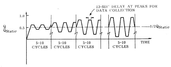
DAY 2 - PROGRESSIVE CYCLING IN TENSION CONSTANT BIAS, INCREASING CYCLIC COMPONENT UNTIL FAILURE OCCURS IN TENSION
