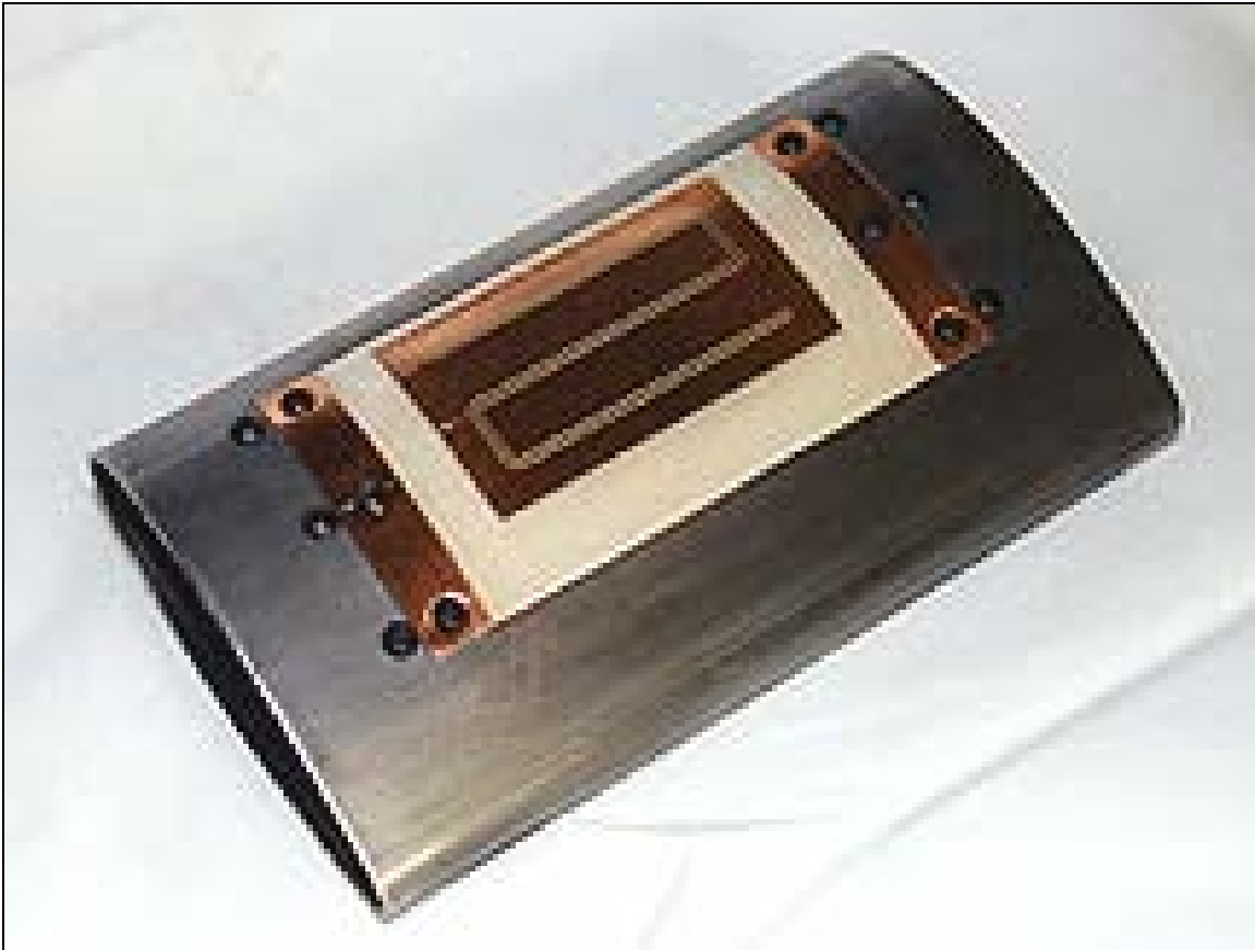
Figure 58. Conformance of Dedicated Electronics' ice detector to icing surface.
