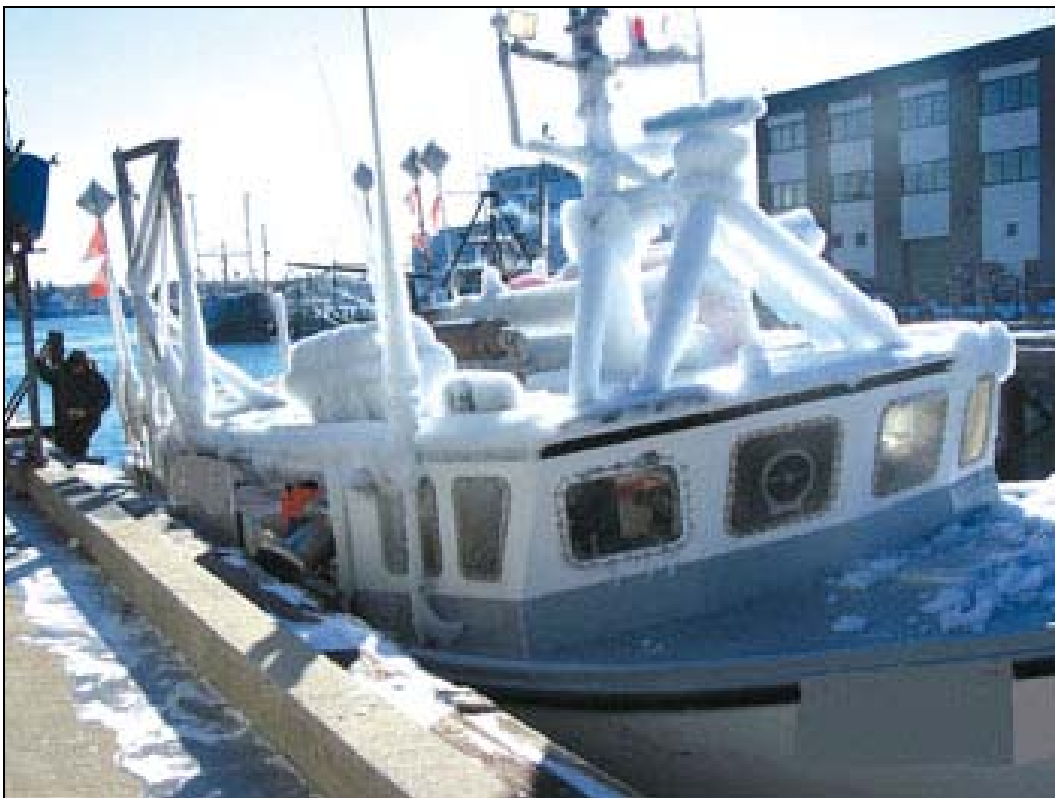
Figure 18. Superstructure ice covering life rafts, antennas, and windows of small trawler-size boat.
