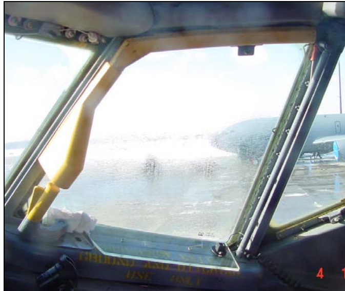
Figure 19. Residues remaining on aircraft windows after testing a non-glycol-based deicing fluid.
