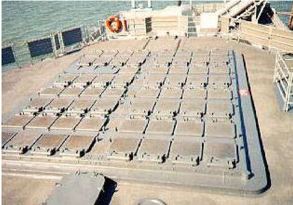
Figure 32. Navy Vertical Launch System with electrically heated door edges.
