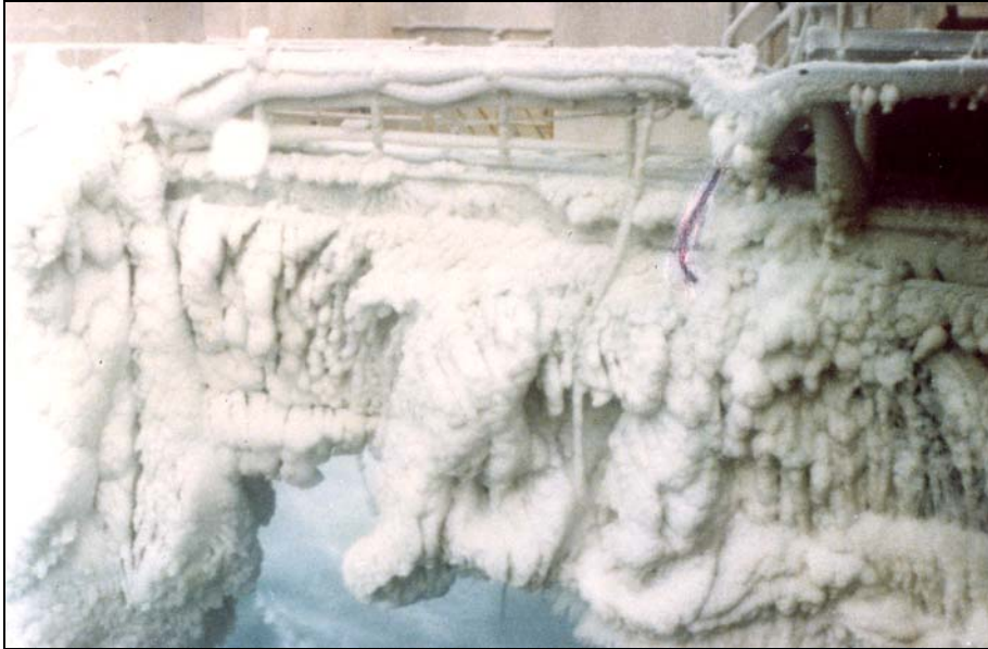
Figure 17. Ice on the upper legs and deck sides of the Ocean Bounty showing probable maximum and thermally limited ice accretion.
