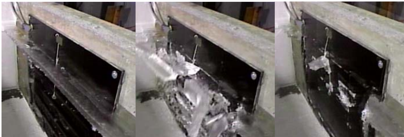
Figure 31. IMS EEDS used for removing ice from a simulated navigation lock wall.
