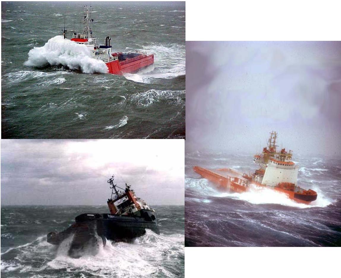
Figure 14. Oil platform supply boats interact actively with the sea, creating abundant spray for superstructure icing.
