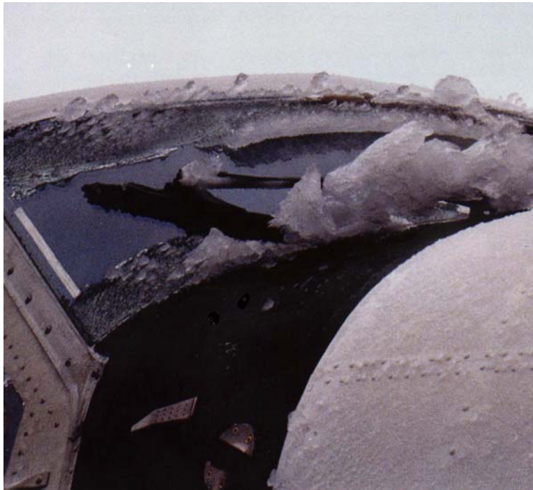
Figure 48. Electrically heated windows on NASA Twin Otter aircraft. The windows are edge-heated: note the vertical heating strip on the extreme right side (left side of image) of the windshield.
