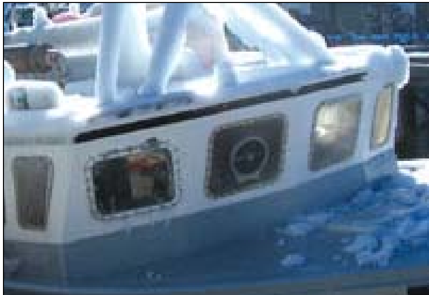
Figure 49. Typical spinning window used to keep ship bridge windows dry and free of ice on Navy ships. Viewed from inside the bridge (top). Spinning window mounted on small supply boat (bottom).
