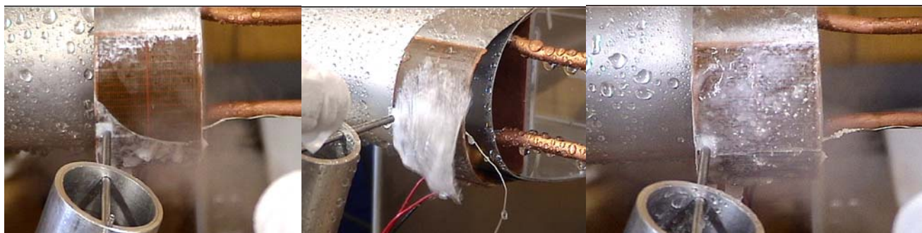
Figure 45. Ice being removed from surface coated with piezometric crystals, left to right.
