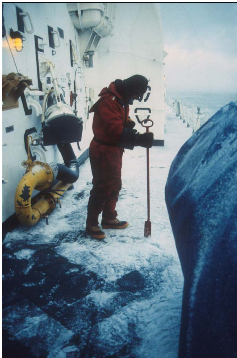
Figure 6. Chipping ice from Coast Guard Cutter deck in Bering Sea, 1990. Mechanical deicing methods damaged deck non-skid material.
