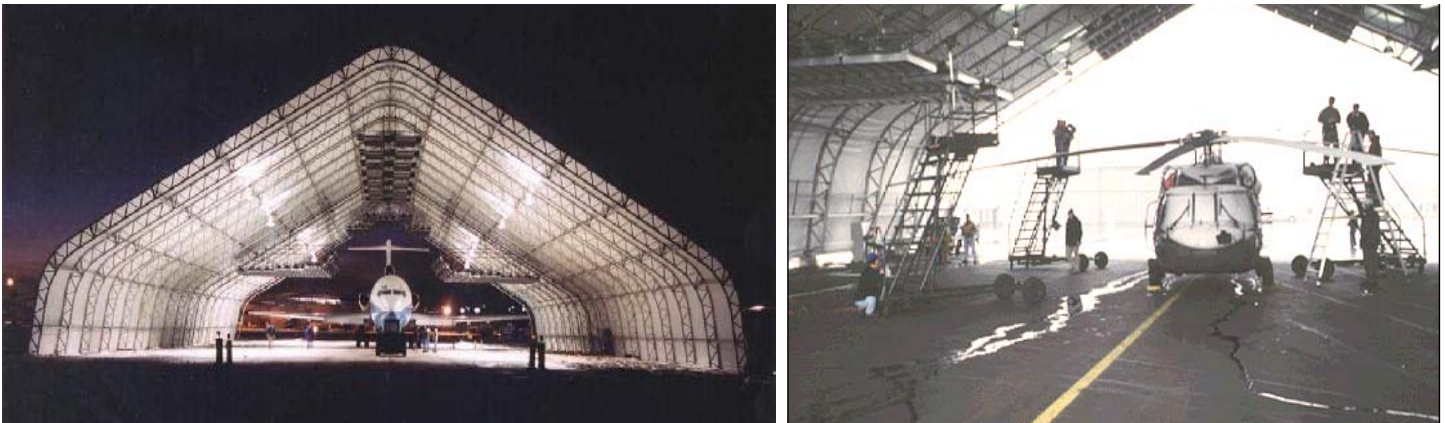
Figure 42. Radiant Aviation Services system for deicing aircraft (left), and in use for experimentally deicing Army helicopters (right).
