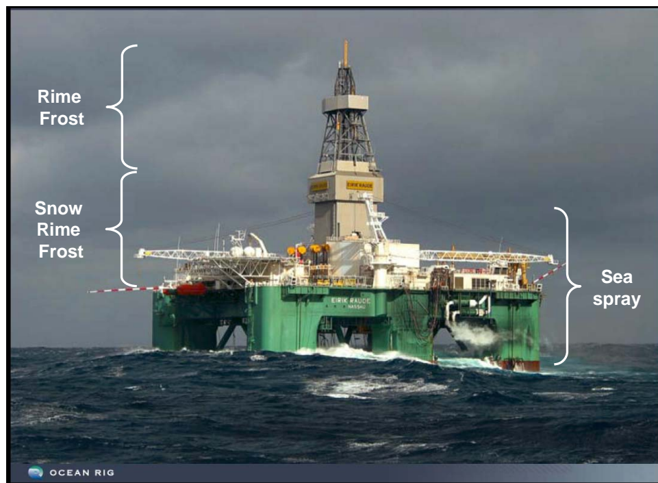
Figure 5. General locations where atmospheric icing (frost, snow, rime, and glaze) and superstructure ice (sea spray icing) would be expected to occur on a drilling platform such as the Eric Raude .
