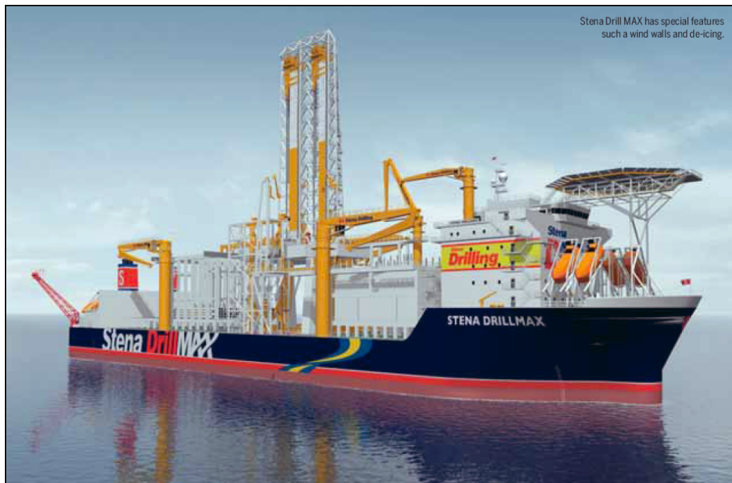
Figure 11. Drill ship Max is designed to minimize cold and icing effects (Pakarinen 2006).
