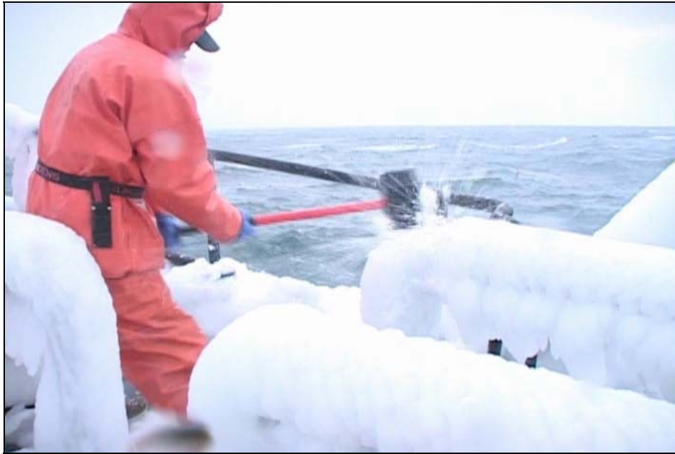
Figure 12. Ice being removed with mallets on crab boat in Bering Sea, 2006.
