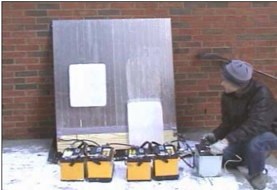
Figure 26. Deicing a metal plate with pulse electrothermal deicing. The ice sheet on the right was released moments before the image frame was acquired.
