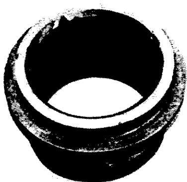
Figure 8: Valve seat cut by fluid erosion caused by over-rotation of the ball valve.
