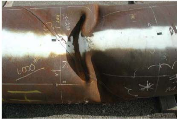
(a) Specimen 1, D/t = 82 , no pressure
