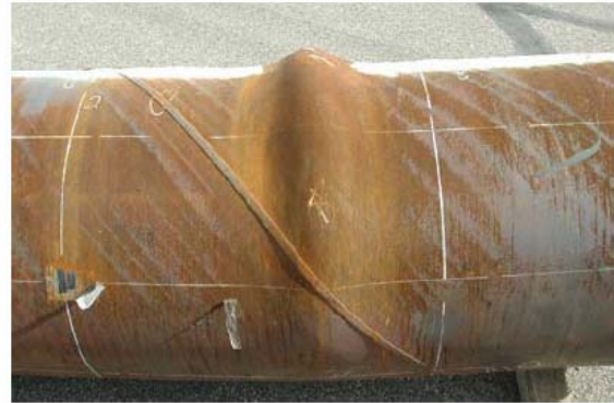
(b) Specimen 2, D/t = 82 , high pressure
