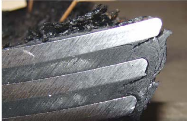
Figure 4.1: Fatigue Crack Initiation in a Failed Flexible Joint Flexible Element [Ref. 20]
