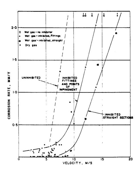
Figure 3.1 Results of Corrosion Measurements by Duncan [7]
