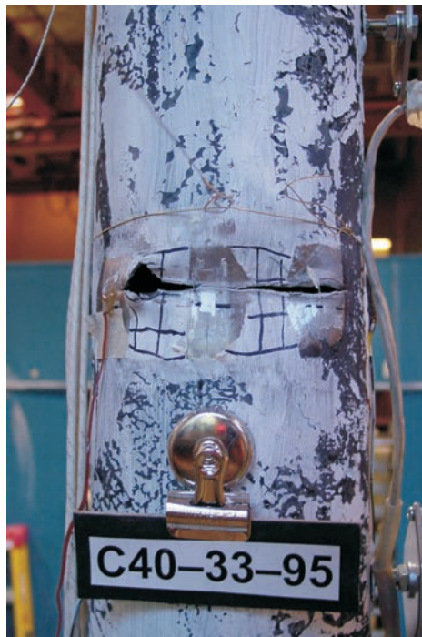
Figure 5.55 Through Thickness Cracking Across Local Buckle (Load Step +4), Specimen C40-33-95
