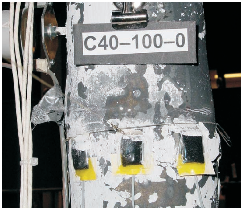
Figure 5.8 Cracking Across Local Buckle (Load Step +10), Specimen C40-100-0
