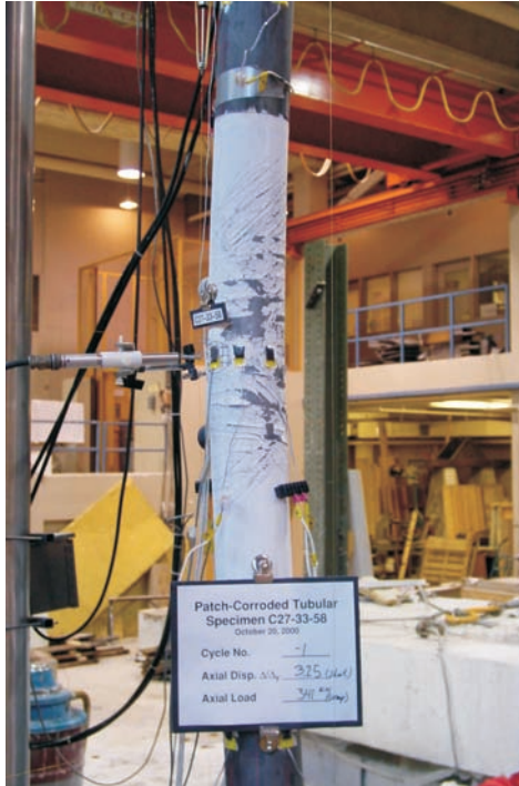
Figure 5.71 Yielding at Mid-height (Load Step -1), Specimen C27-33-58
