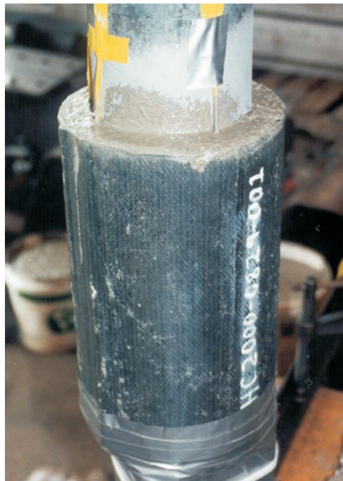
Figure 4.27 Local View of Specimen C40-00-95-RC with Composite Repair Sleeve Installed
