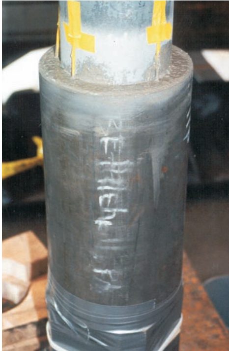
Figure 4.26 Local View of Specimen C40-00-95-RS with Steel Repair Sleeve Installed
