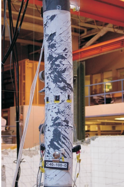
Figure 5.5 Side View of Yielding at Mid-height (Load Step -1), Specimen C40-100-0
