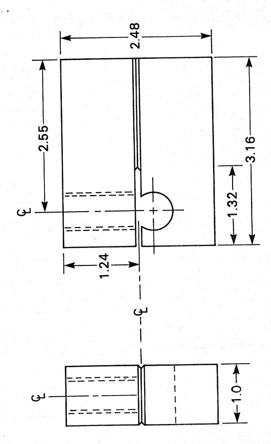
Figure 1 – Configuration of the 1T WOL fracture mechanics test specimen.
