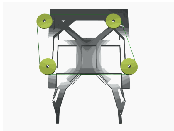
Figure 9.6 – 60" OD Diamond Wire Cutting Tool
