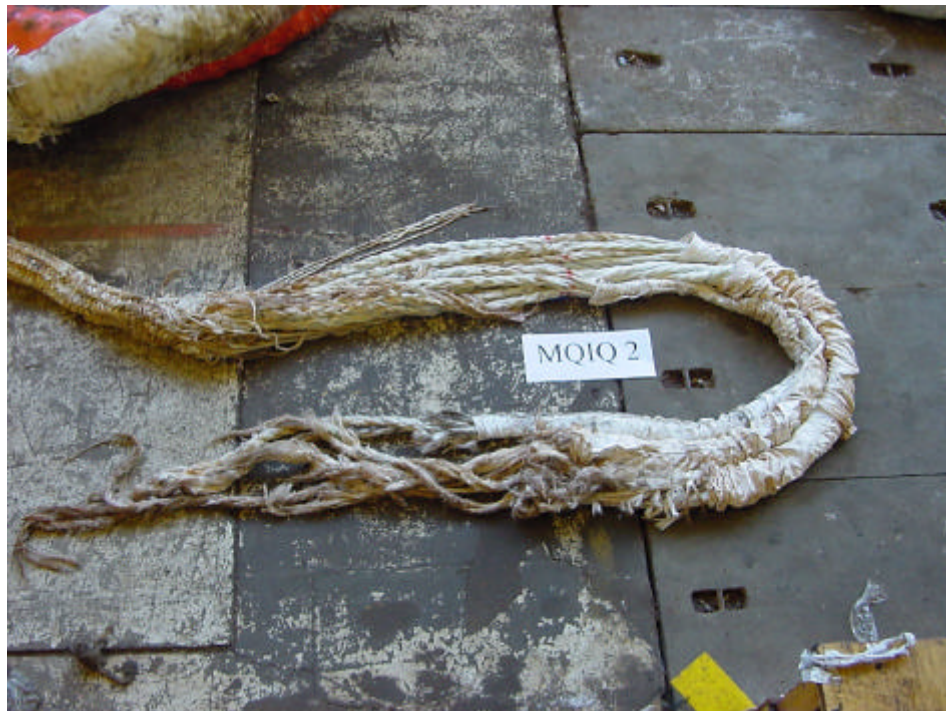
Figure 8.10 MQIQ 2 – Failure Region Resulting From Break Test
