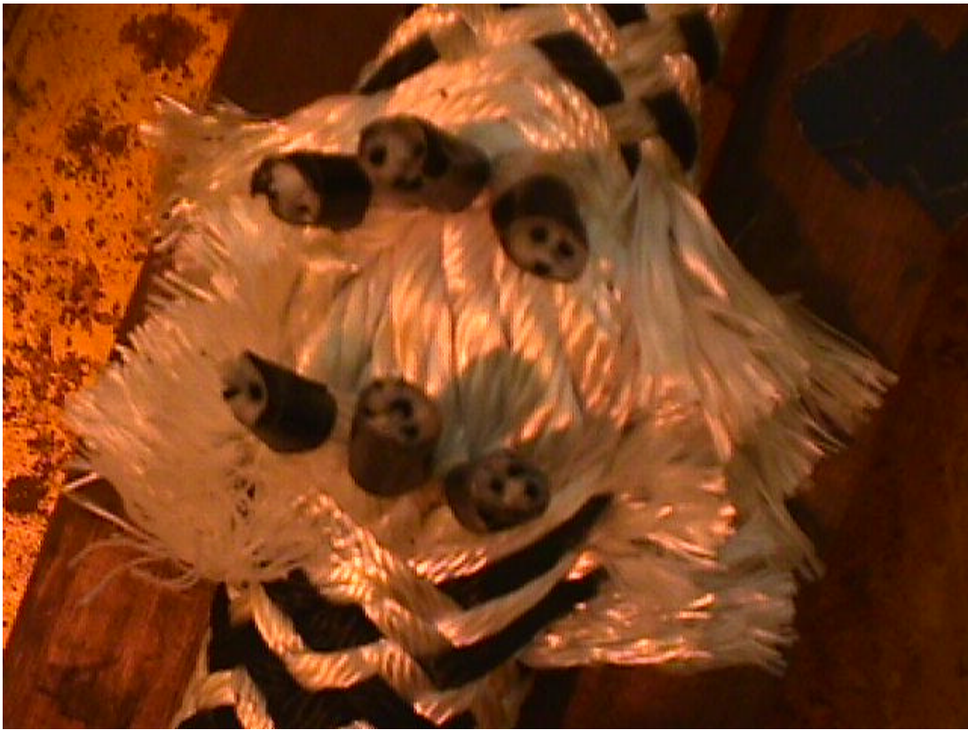
Figure A5. MQDE 4 With 3 Subropes Cut
