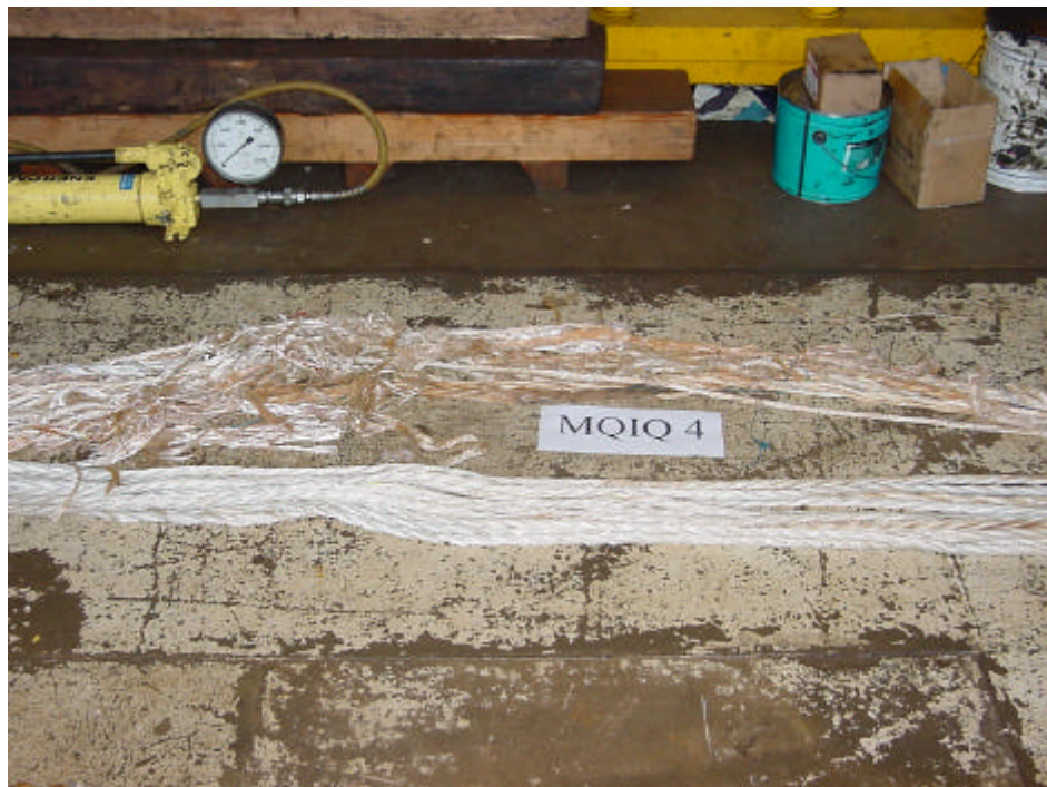
Figure 8.18 MQIQ 4 – Failure Region Resulting From Break Test
