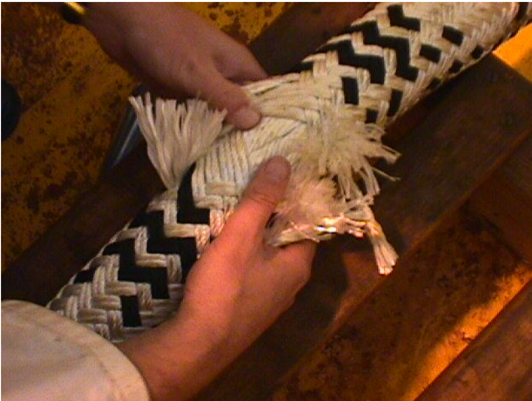
Figure A2. Further Removal of Jacket
