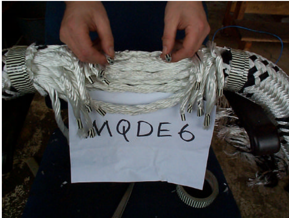
Figure 7.26 MQDE 6 – Nine Subropes Cut
