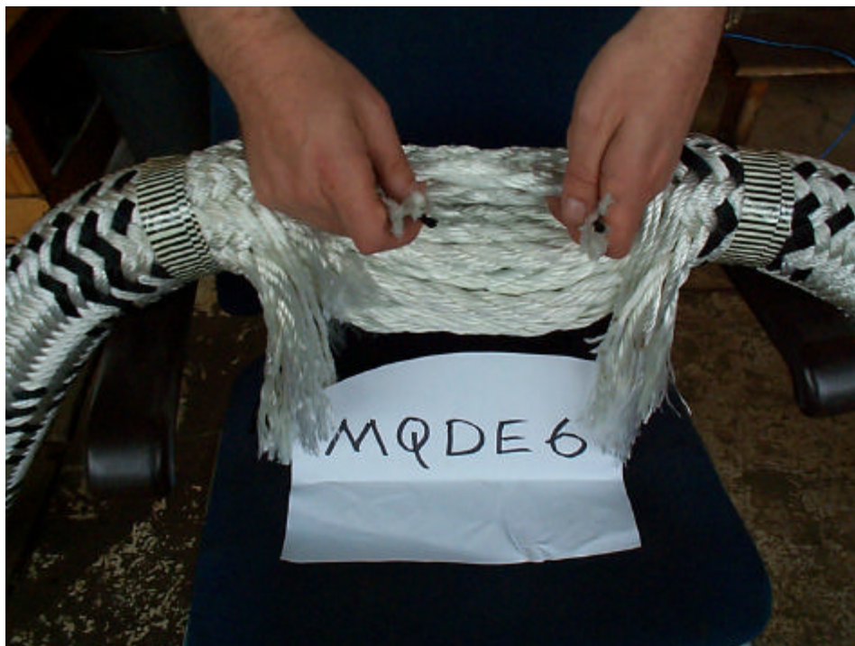
Figure 7.25 MQDE 6 – First of Nine Subropes Cut
