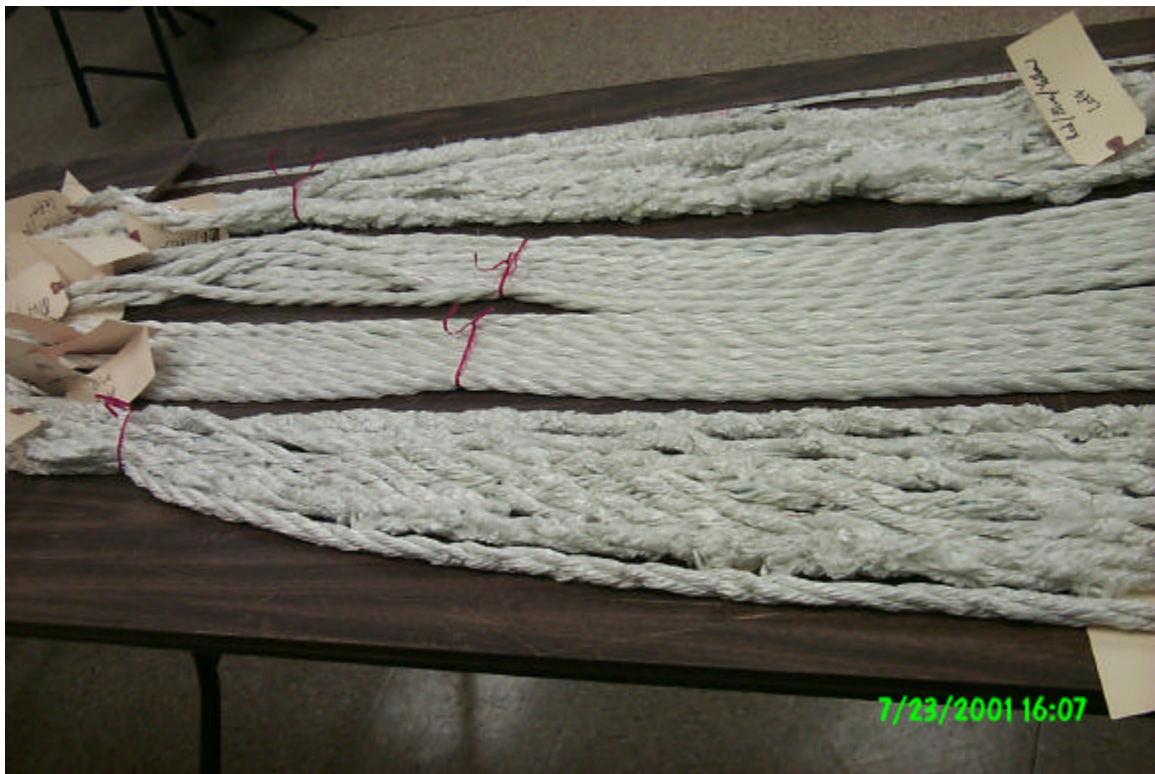
Figure C-5. Close-up of SES 2 Showing Outer Bundles Containing Subropes Affected By Bunching Up Under the Jacket.
