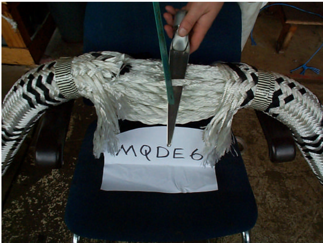
Figure A8. Cutting a Subrope.
