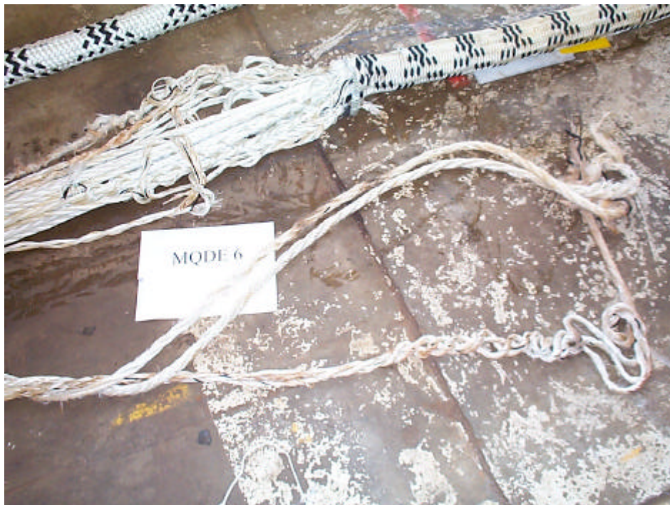
Figure 7.27 MQDE 6 – Failure Region Resulting From Break Test
