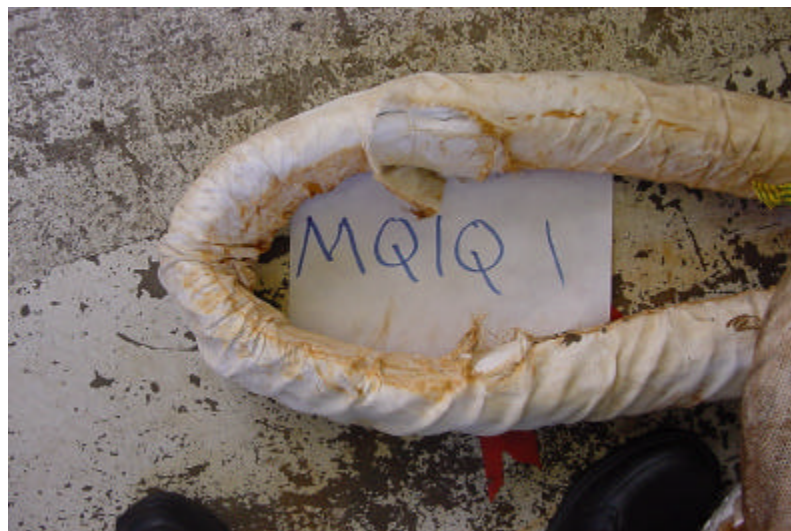
Figure B14. Photo of Wear in Outer Cover at Upper and Lower Tangent Points.
