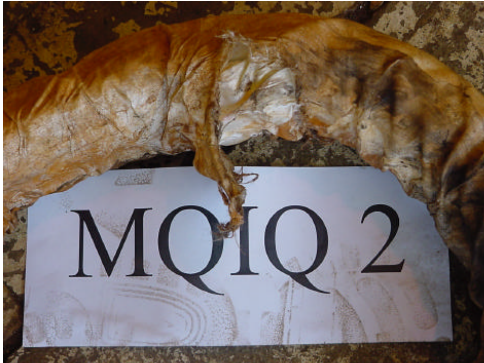
Figure 8.11 MQIQ 2 Wear of Outer Cover at Point Where Rope First Makes Contact with Spool (Tangent Point)
