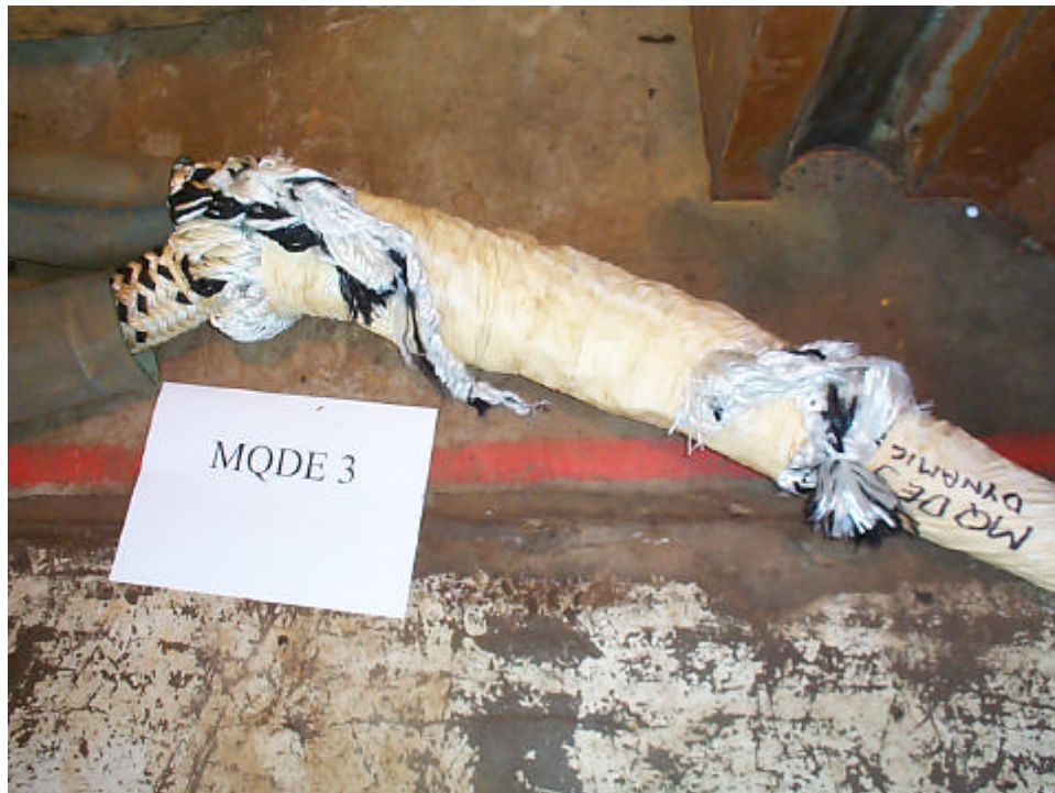
Figure 7.19 MQDE 3 – Failure Region Resulting From Break Test
