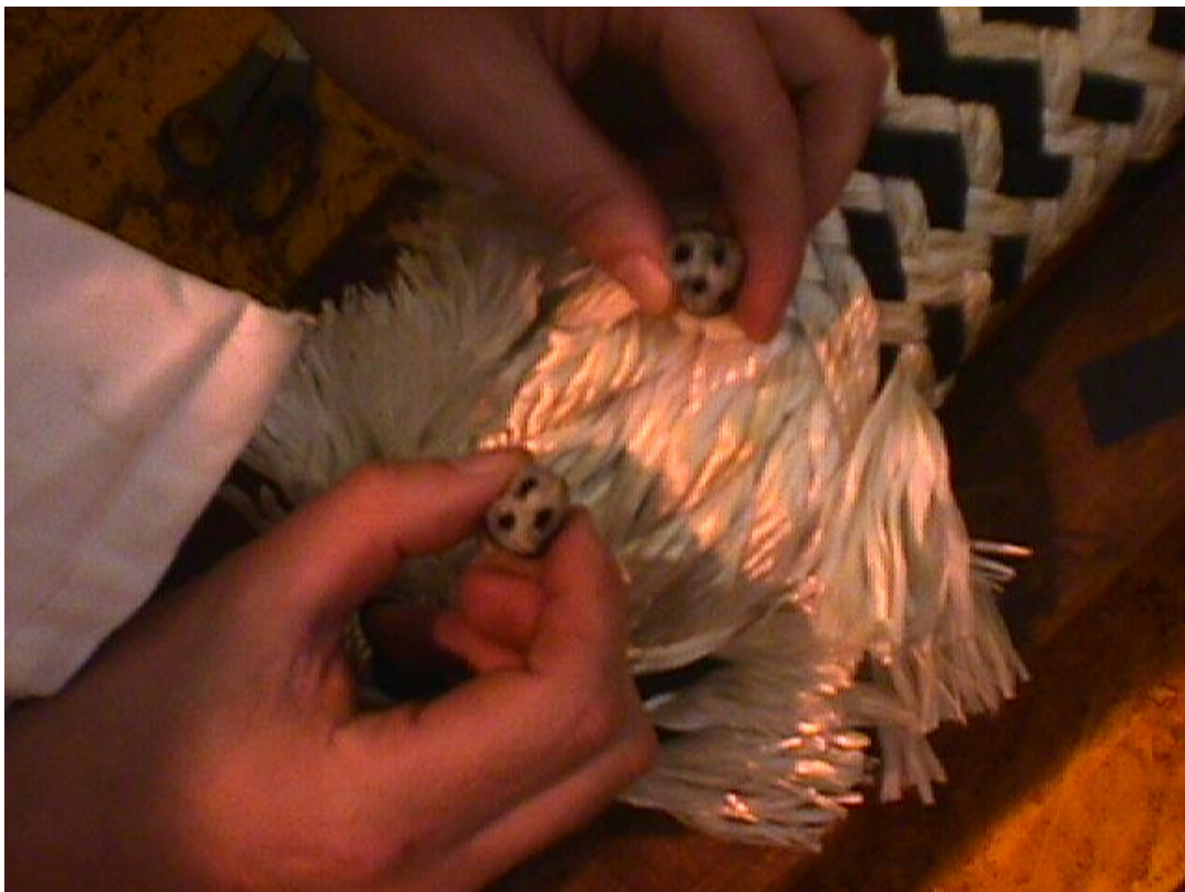
Figure A4. Cut Subrope Showing Black Marker in Each Element.
