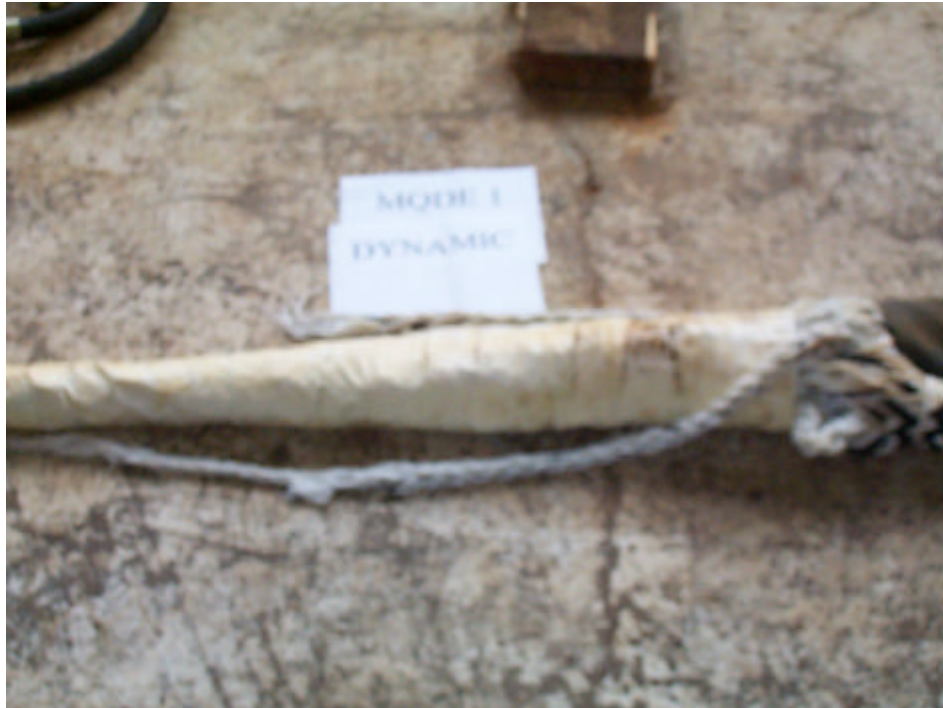
Figure 7.18 MQDE 1 – Failure Region Resulting From Break Test
