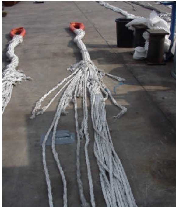
Figure B26. Failure Photo for SES 6.
