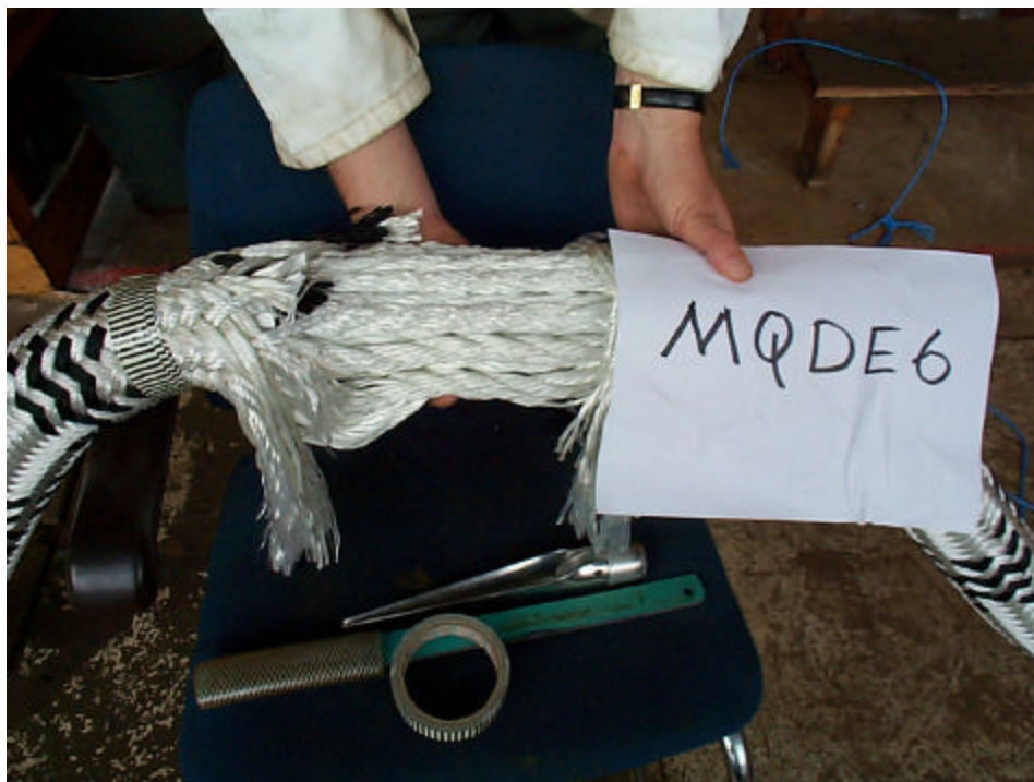
Figure 7.23 MQDE 6 – Jacket Removed
