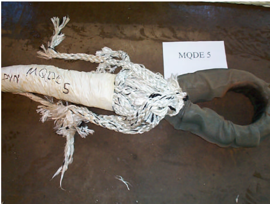
Figure 7.21 MQDE 5 – Failure Region Resulting From Break Test
