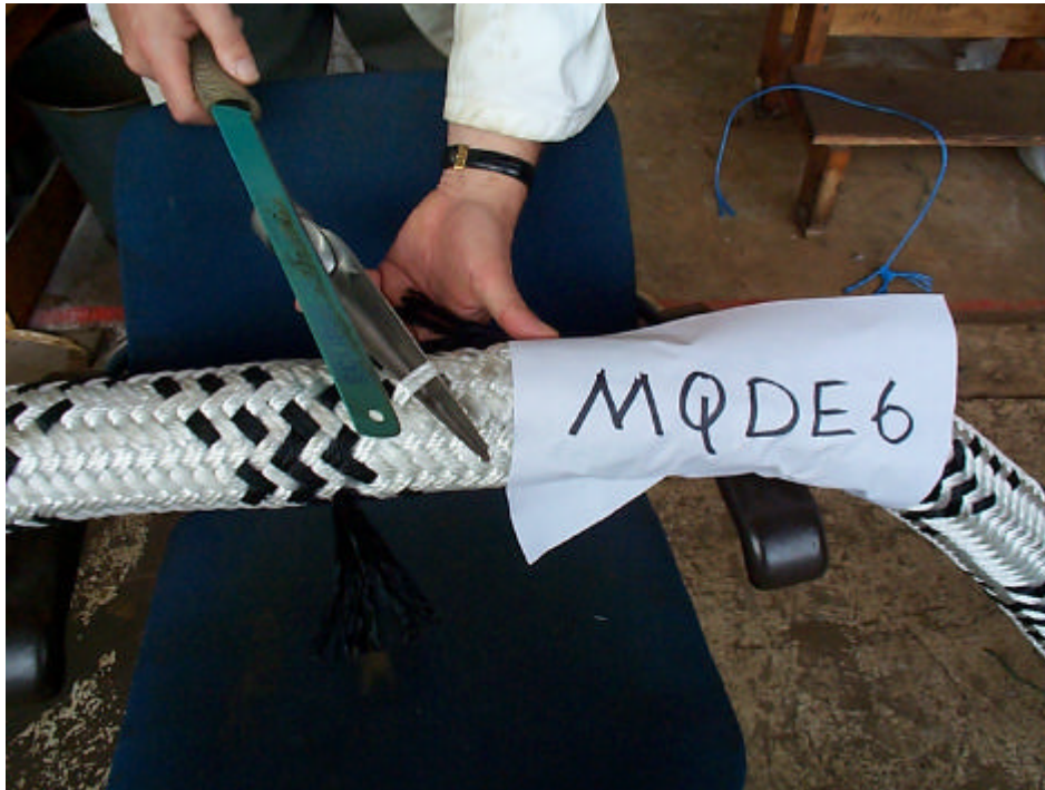
Figure 7.22 MQDE 6 – Commencement of Jacket Removal
