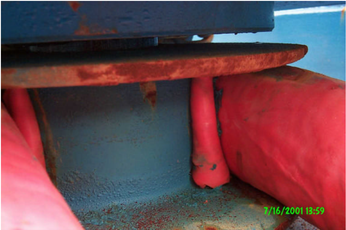
Figure C-3a. Coating Extrusion Damage Caused by Thimble Loading.
