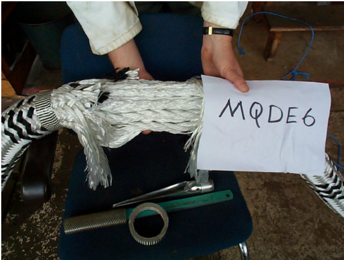
Figure A7. Jacket Removed.
