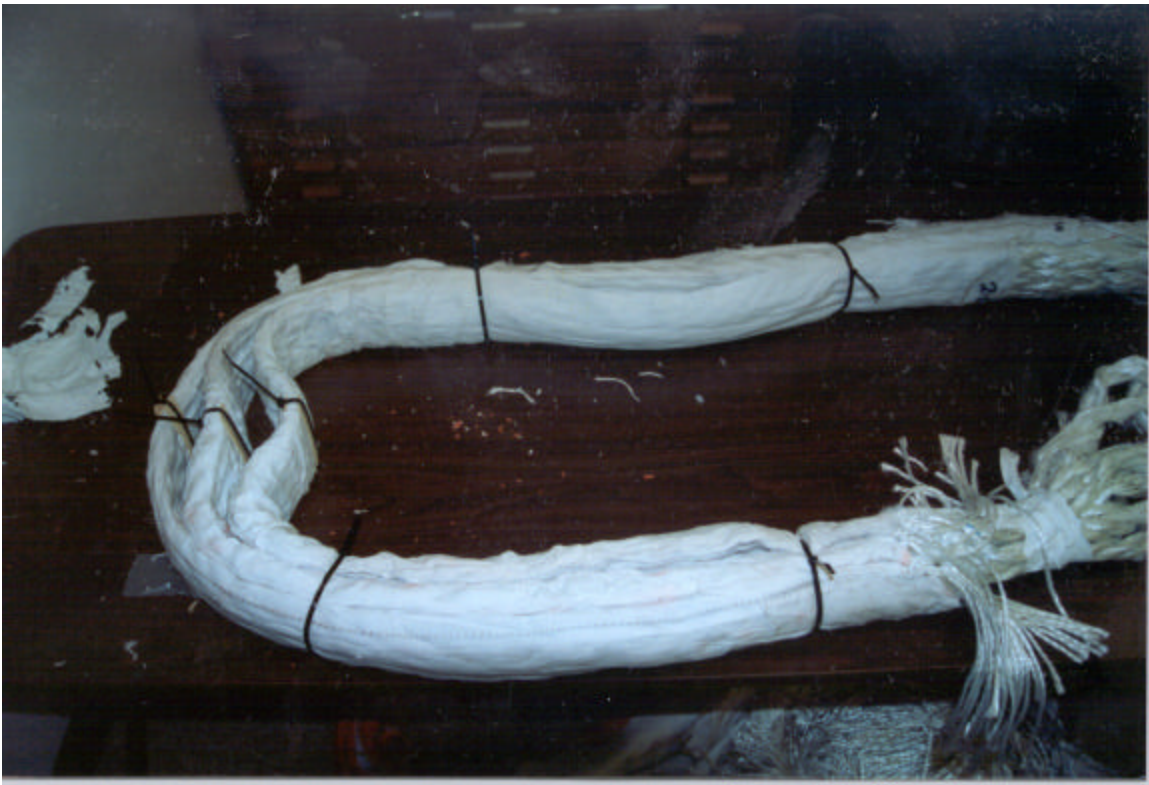
Figure C6. SES 2 Eye Splice Region with Outer Jackets Removed. Note Subrope Bundles in Three Layers.
