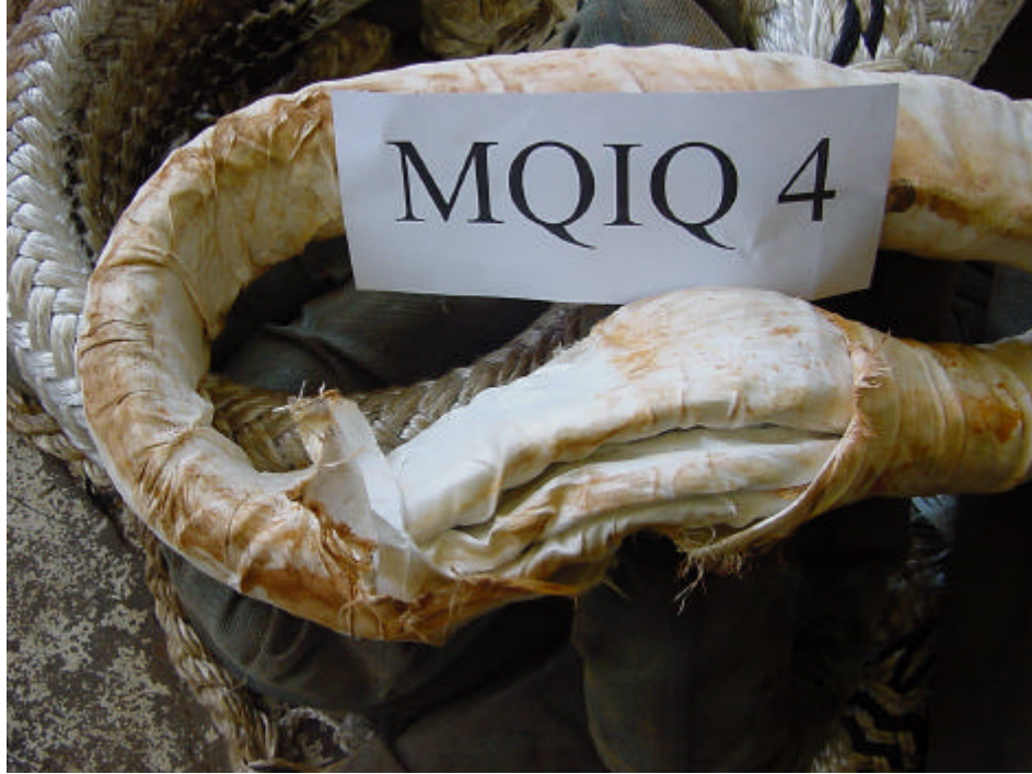
Figure 8.19 MQIQ 4 Wear of Outer Cover at Point Where Rope First Makes Contact with Spool (Tangent Point) Fixed End Eye
