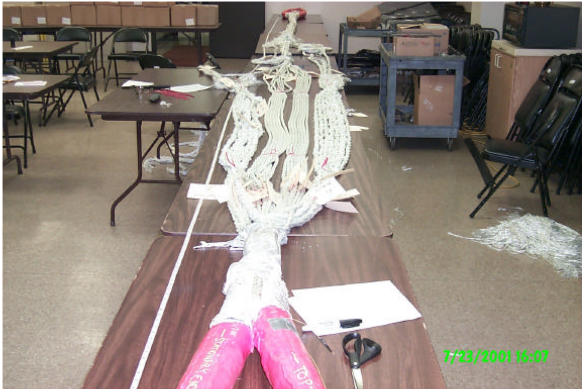
Figure C4. Sample SES 2 with Jacket Removed, Showing Inner Two Bundles of Undamaged Subrope, and Outer Two Bundles of Broken/Cut Subrope.
