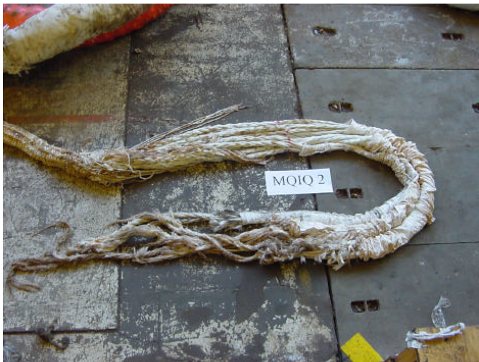
Figure B15. Failure of MQIQ 2 at One of the Eyes.
