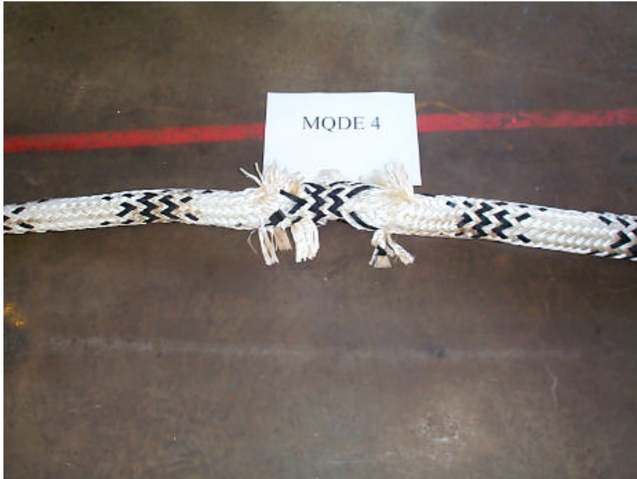
Figure 7.20 MQDE 4 – Failure Region Resulting From Break Test
