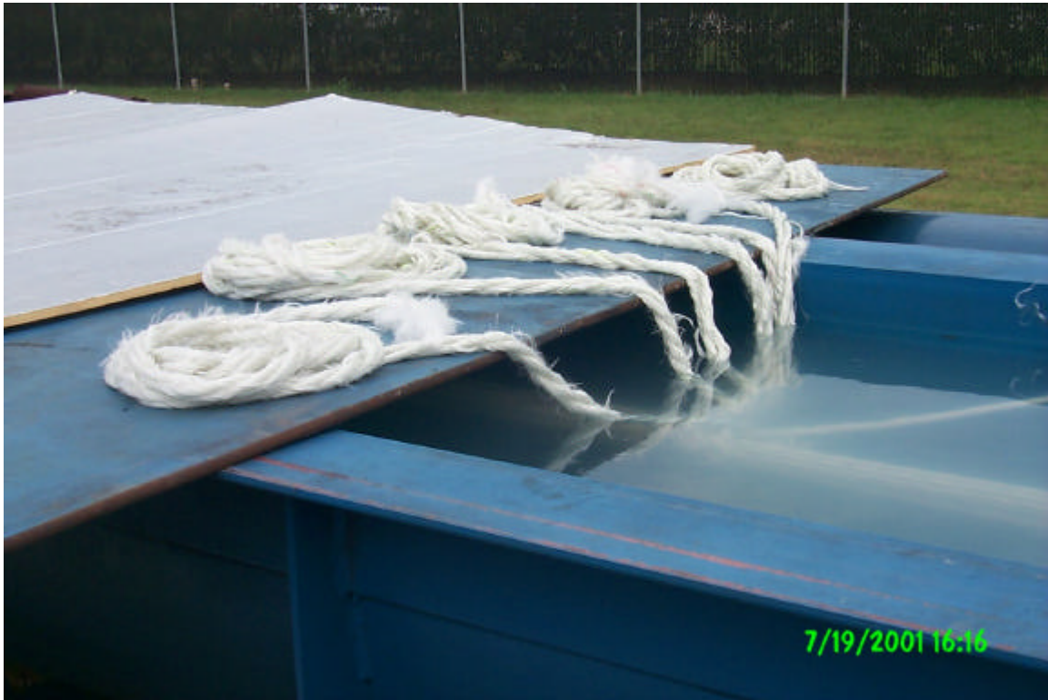
Figure C-1. Broken/Cut Subropes Found After Test SES 2 Stopped. Note Tensioned Ropes in the Water.
