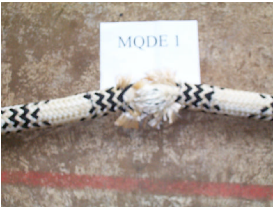
Figure 7.17 MQDE 1 – Induced Damage Region After Break Test
