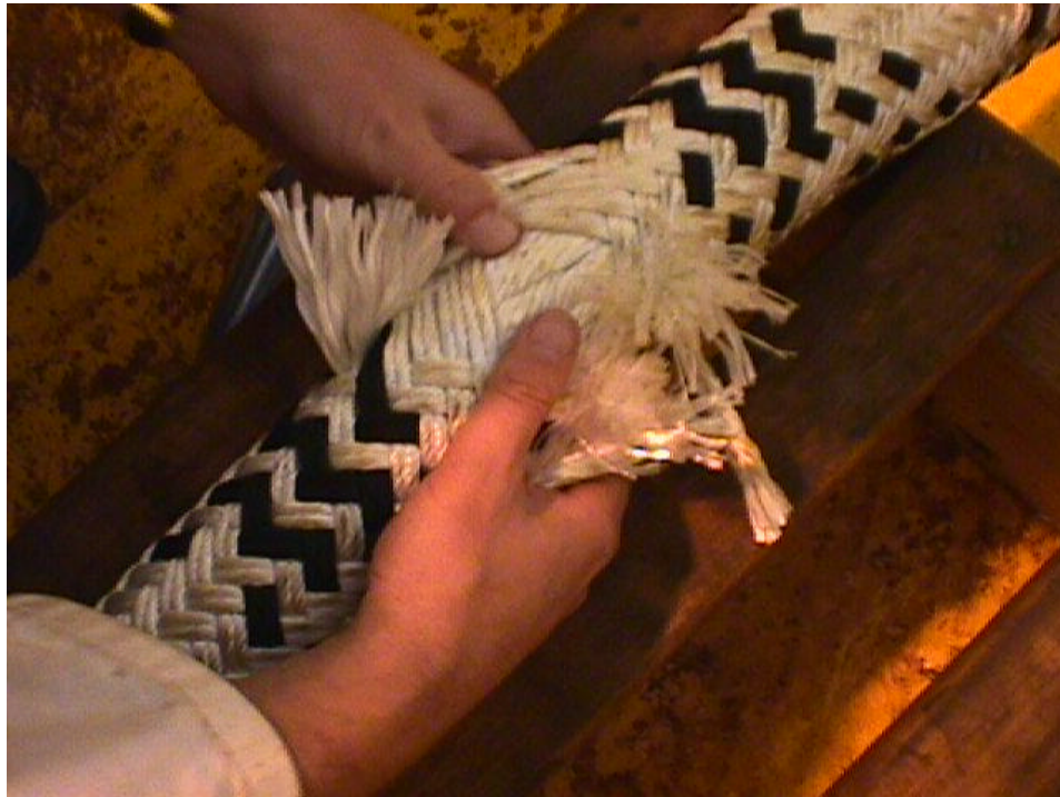
Figure 7.13 MQDE 1 – Removal of Jacket Continued
