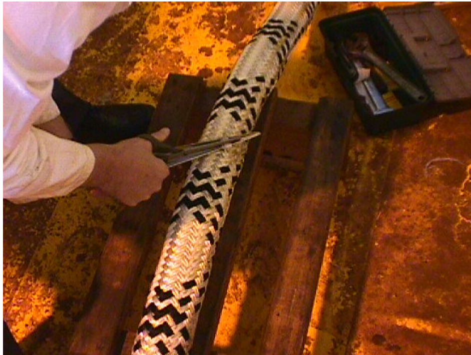
Figure 7.12 MQDE 1 – Removal of Jacket
