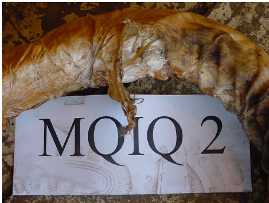
Figure B16. Wear of Eye at Opposite End of MQIQ 2.
