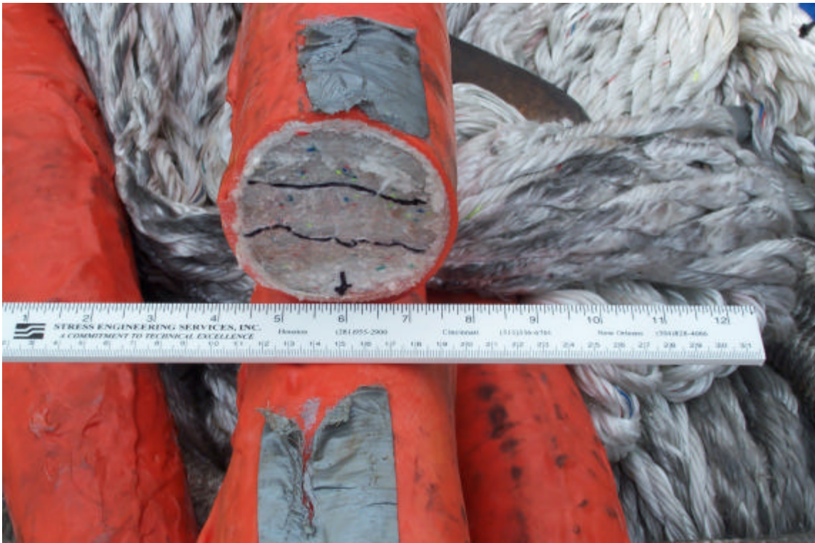
Figure C8. Cut Through Eye Cross Section Showing Three Layers.
