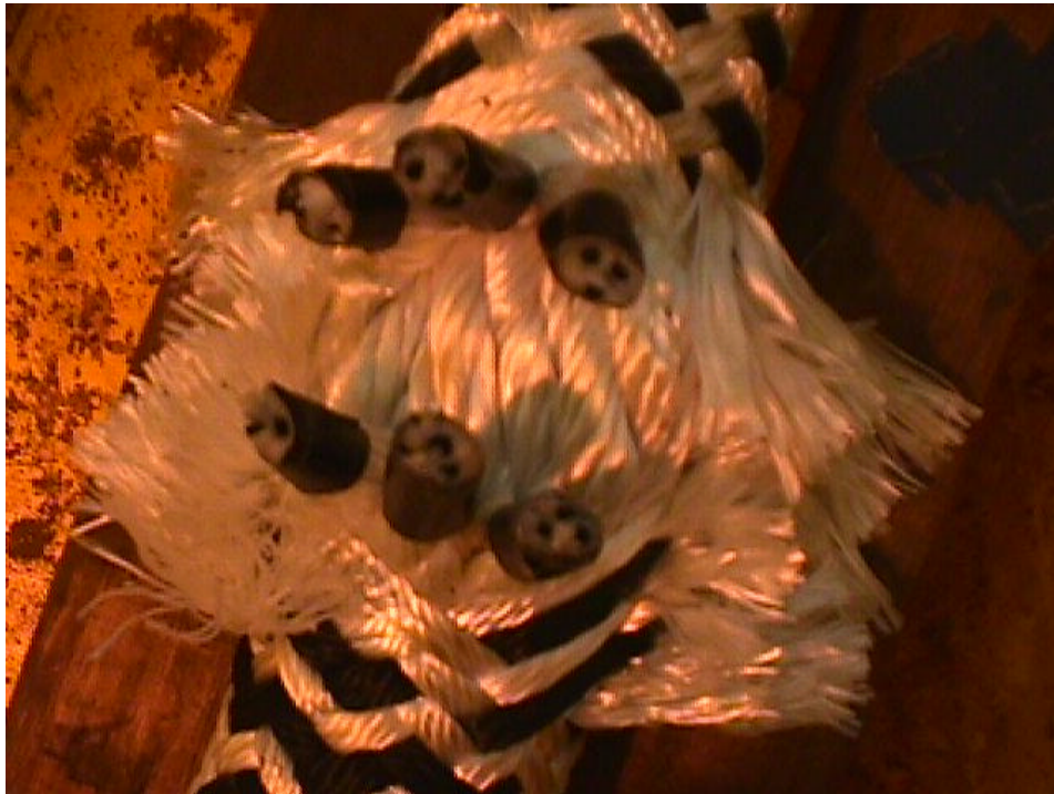
Figure 7.16 MQDE 1 – All Three Subropes Cut
