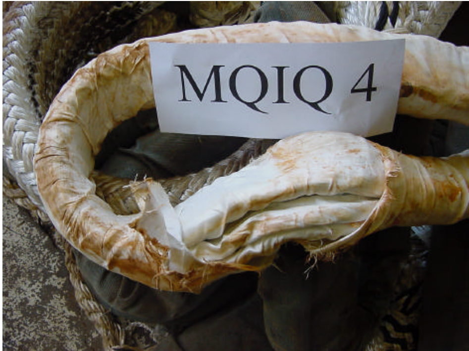
Figure B20. Wear of Outer Cover of Splice in MQIQ 4.
