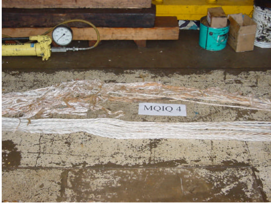
Figure B19. Failure of MQIQ 4 in the Center Section.
