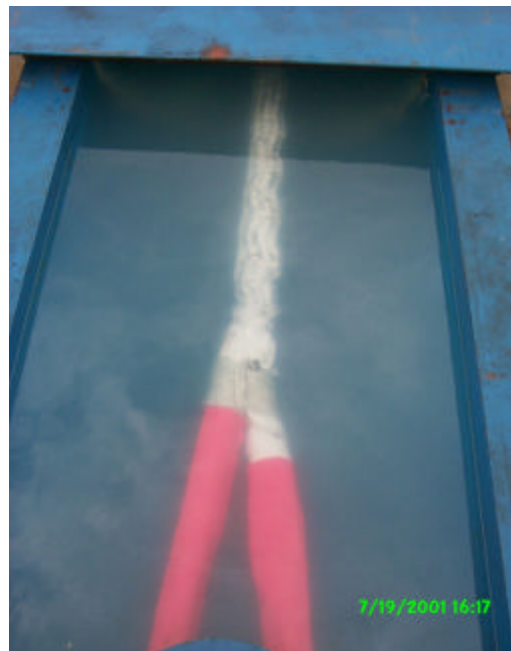
Figure B12. Photograph of Splice Rotation on SES 2. Note Lack of Symmetry.
