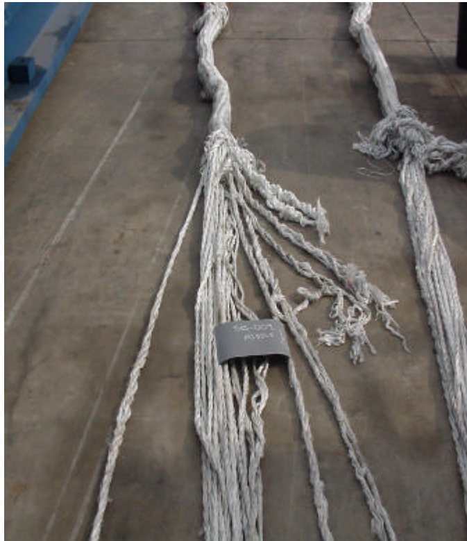
Figure B24. Failure of SES 4.
