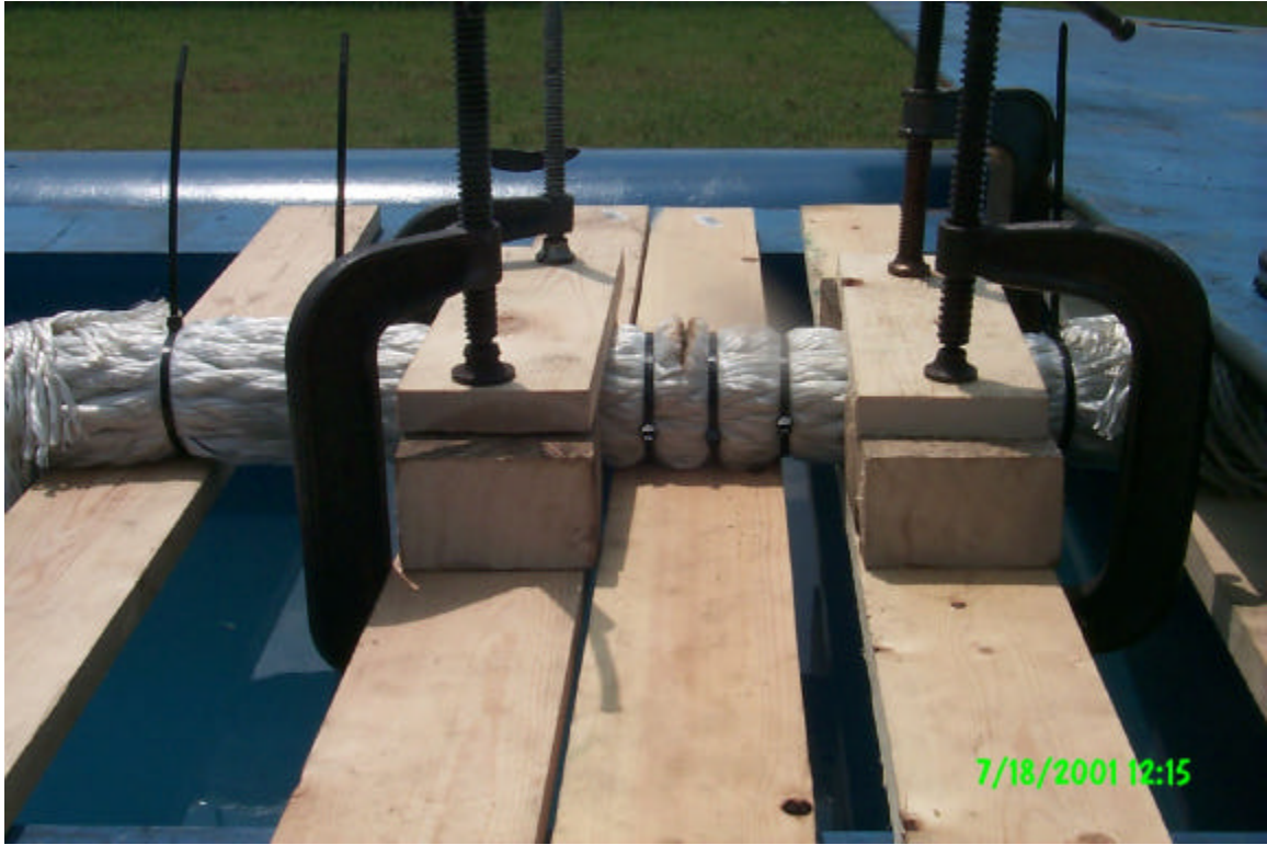
Figure B5. Close-Up of the Cut Rope. Note Raised Cut Region.
