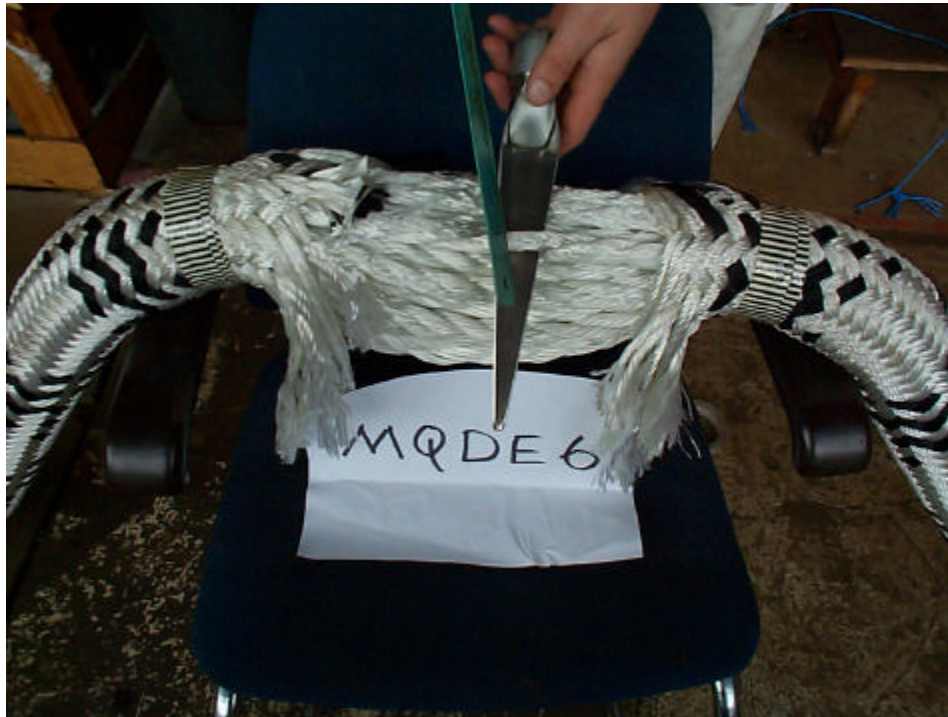
Figure 7.24 MQDE 6 – Cutting of Subrope
