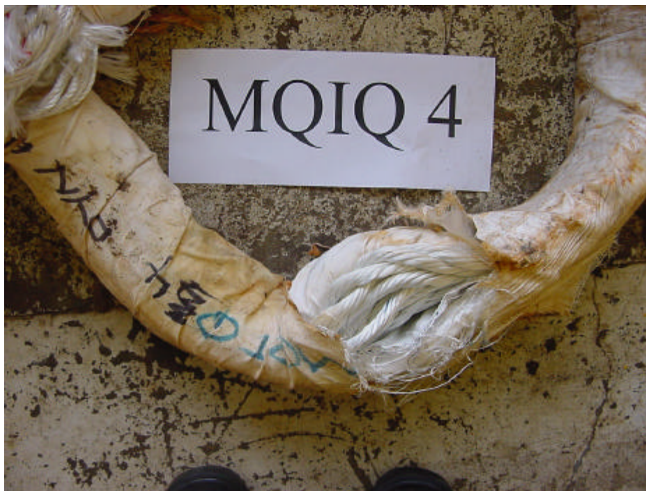
Figure B21. Eye Wear at Other End.
