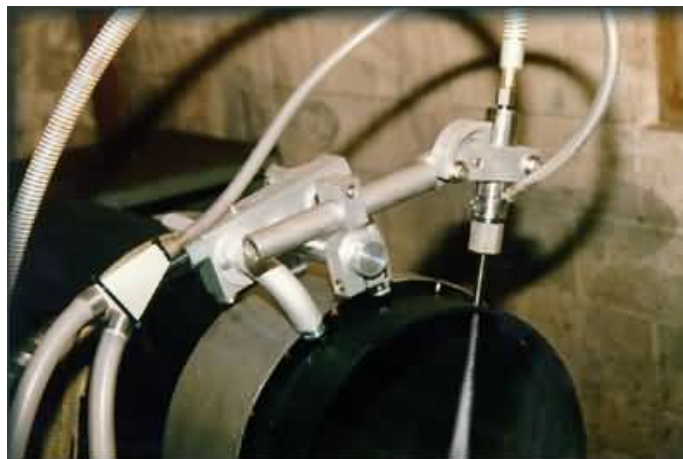
Figure 6.1: Abrasive water-jet systems
