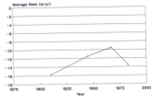
FIGURE 27.—Average gulfside rate of change along the Caminada-Moreau Headland between 1887 and 1988.
