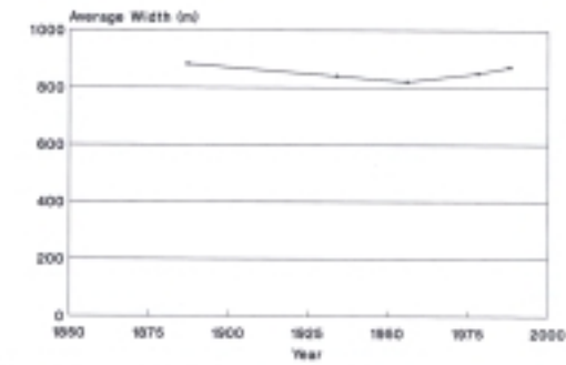
FIGURE 35.—Average barrier width of Grand Isle between 1887 and 1988.
