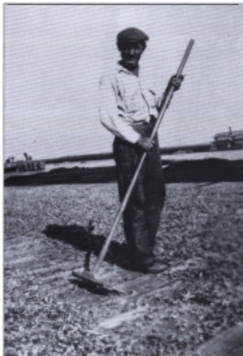
To insure uniform dehydration, the shrimp were spread evenly over the cypress platform's surface with wooden rakes, no date: (Louisiana State Library, Louisiana Collection, WPA Photographic Archives)
