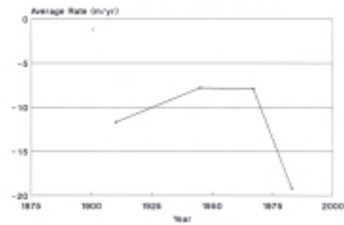
FIGURE 5.—Average gulfside rate of change along Isles Dernieres between 1887 and 1988.
