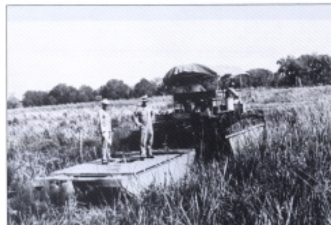
Seismic crews used marsh buggies to run their profiles, ca. 1950: (Louisiana Department of Wild Life and Fisheries, Photographic Archives)
