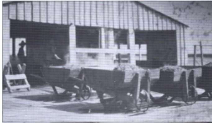
Shrimp used in the shrimp-drying business were boiled in a hypersaline solution. When removed from the vats, the shrimp were taken by wooden wheelbarrows to the platform's drying area, ca. 1920: (Randolph Bazet Collection, Houma, Louisiana).
