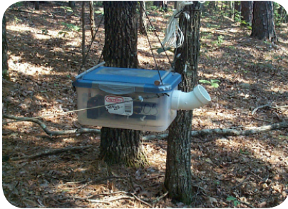
Above: Anabat device for recording bat calls in protective container in forested setting.
