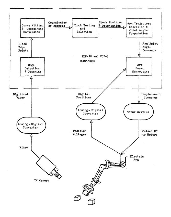
Figure 2 The Initial Block-Stacking System
