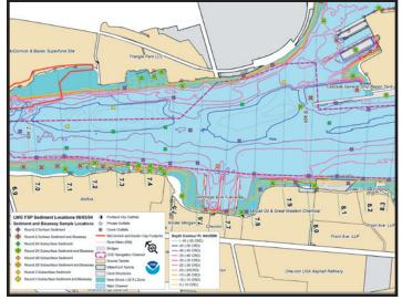
This figure shows a small section of the field sampling plan that was developed using the watershed project. Many factors influenced the sampling plan, including the type and value of the various habitats in the river, the depth of the water, the location of existing data, and the proximity of known or suspected sources of contamination. The watershed project allowed us to integrate all these factors and identify data gaps where additional samples were needed.
