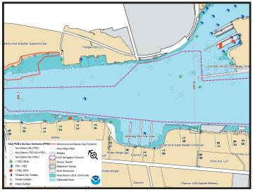
This figure shows total PCB concentrations in surface sediments. The red dots represent sediment samples from numerous studies where toxicity to benthic organisms is likely, due to total PCB concentrations that exceed screening guidelines. Analyses like this one highlight areas that require further study, and may be used to help identify possible sources of contamination in the river
