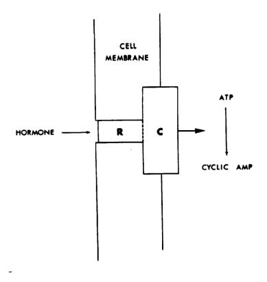
Fig. 1: 1967 Conceptualization of an hormone-sensitive adenylyl cyclase. The enzyme is modelled after the multisubunit enzyme aspartic transcarbamo-ylase, in which the catalytic unit (adenylyl cyclase proper) would be under the regulation of allosteric ligands (hormones, neurotransmitters) by interacting with specific sites located on regulatory subunits (receptors). (From Robison et al., 1967).
